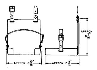
Metal tray for carrying Sensitive Research Instrument Corp. Model "Bellud" milli-voltmeters and Weston Model 931 voltmeters while taking battery readings. Equipped with leather straps for fastening around the neck and for securing the meter to the tray.
