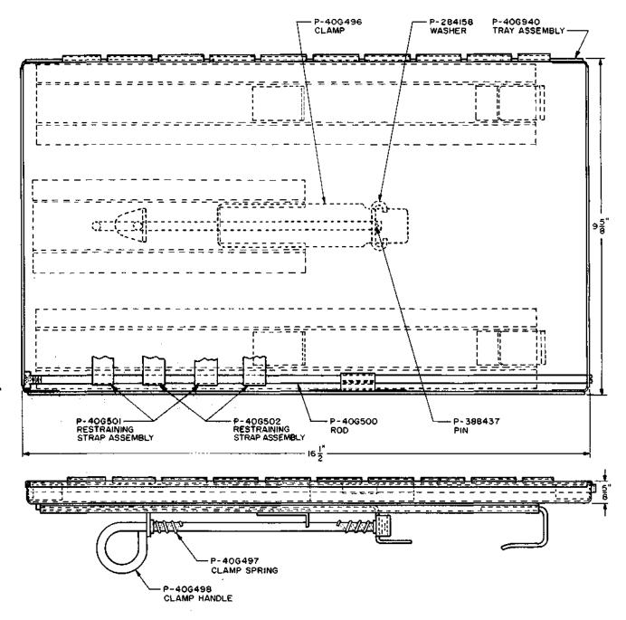
Designed to hold a variety of ammeters, ohmmeters, and voltmeters used in Central Offices. Intended for attachment to the steps of rolling ladders.
