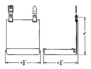
Metal tray for carrying a Weston Model 280 or 281 voltmeter while taking battery readings. Equipped with leather strap for fastening around the neck.
