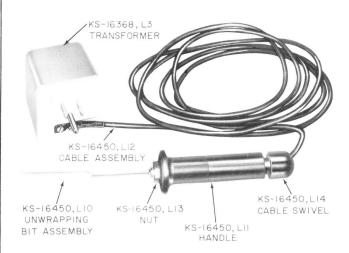
A heated wire-unwrapping tool for use in loosening and removing soldered-wrapped connections of 22-, 24-, and 26-gauge wires.
