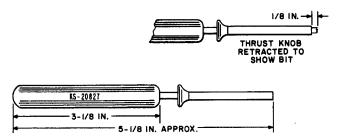
A manually operated tool, with an insulated retractable sleeve, used primarily to unwrap and remove solderless-wrapped connections of 22-, 24-, and 26-gauge wires.
