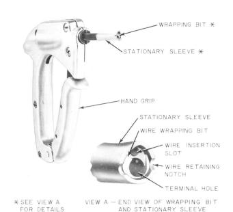
→A manually operated tool which is primarily used for making solderless-wrapped connections. Wrapping bits and stationary sleeves must be ordered separately for use with this tool. Refer to Section 074-520-101 for the wrapping bits to be used with this wire-wrapper. Refer to Section 074-775-101 for the wrapping sleeves to be used with this wire-wrapper. ←
