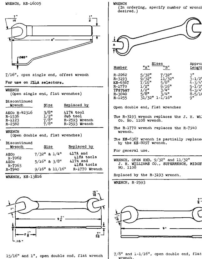
For use on 168B, 170A, and 171A precision type interrupters for loosening clamping nuts at end of cam shaft.
