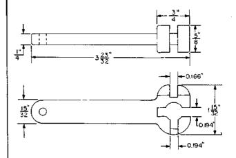
Wiper-shaft aligning wrench
