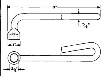
5/8-inch offset hex. socket wrench. For use on precision-type interrupters, gear reduction drives, and friction roll drives.
