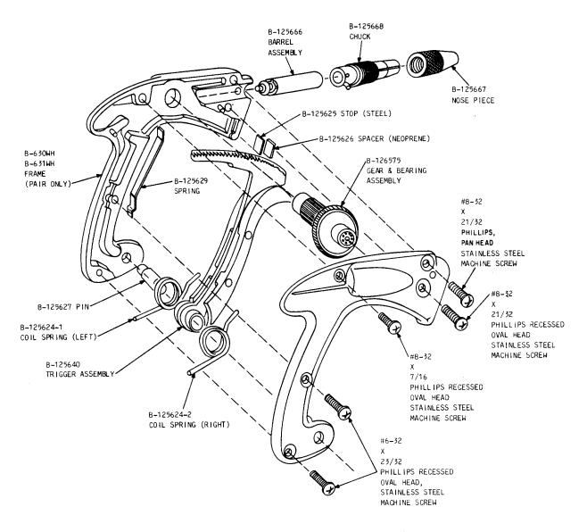
Fig. 2—KS-16363 Wire-Wrapping Tool—Exploded View
