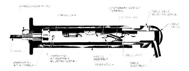
Fig. 2—Cross Section of Handle Assembly for KS-16450 L1 Wire Unwrapping Tool
