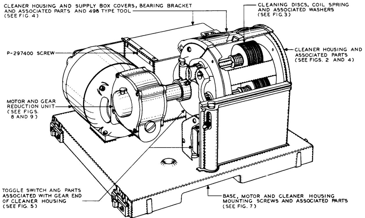
Fig. 1 - Nos. 497A, 497B, and D-159798 Tools (Portable Plug Cleaning Machine)
