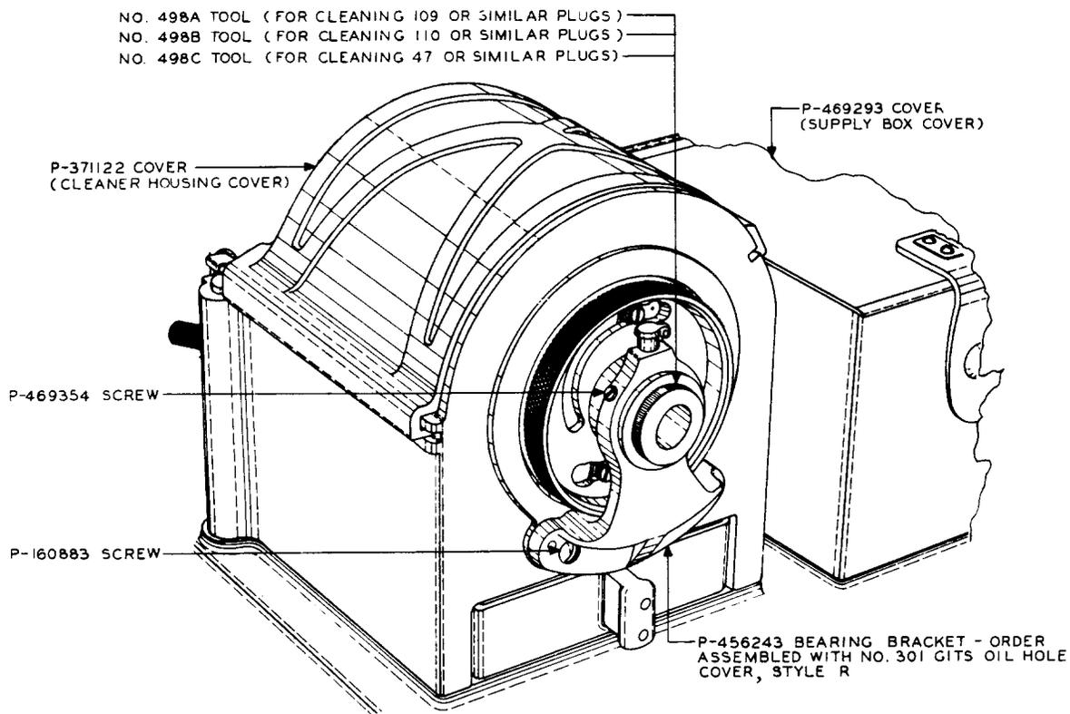
Fig. 4 - Cleaner Housing Cover, Supply Box Cover, Bearing Bracket and Associated Parts, and 498-type Tool
