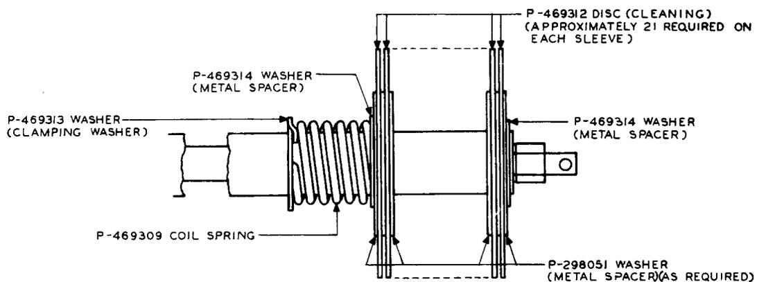
Fig. 3 - Cleaning Discs, Coil Spring, and Associated Washers
