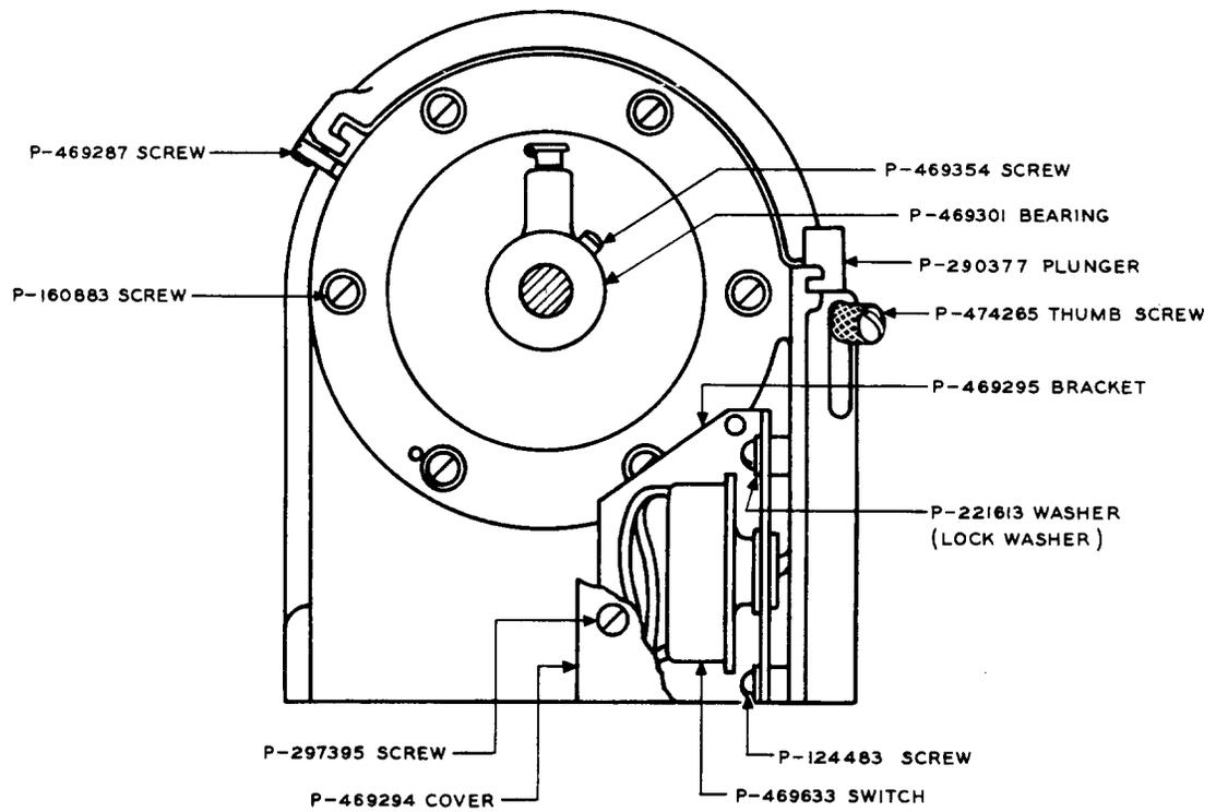
Fig. 5 - Toggle Switch and Parts Associated with the Gear End of the Cleaner Housing
