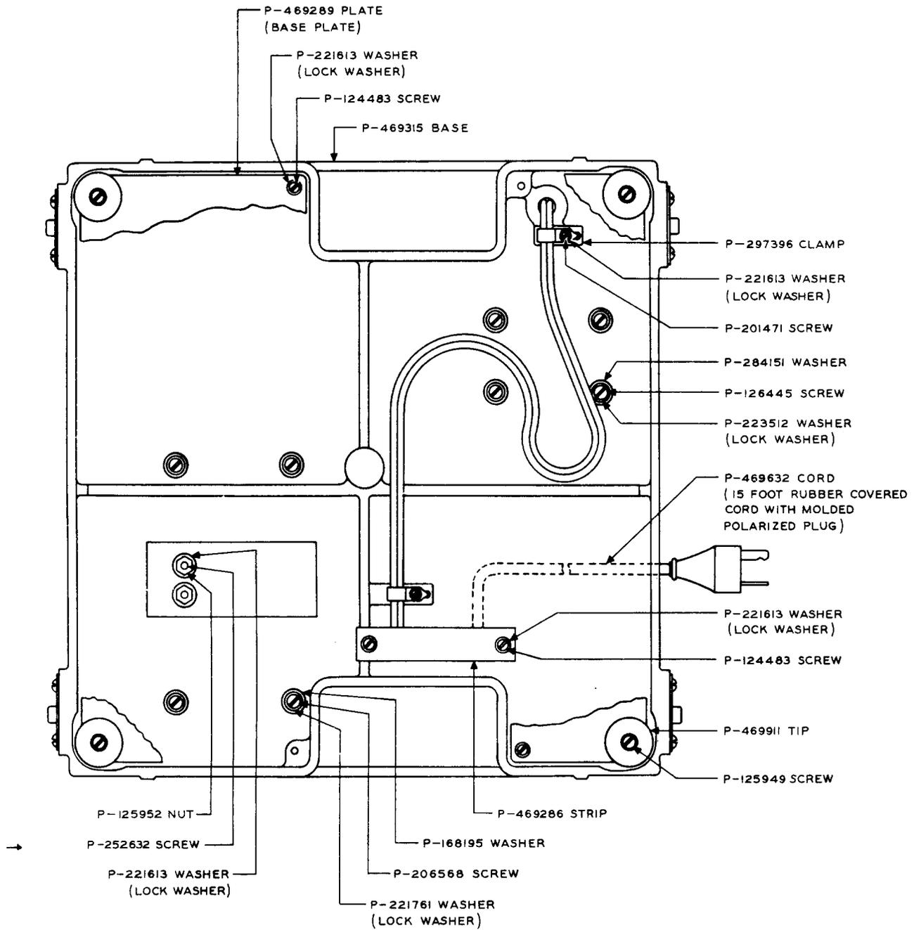
Fig. 7 - Base, Motor, and Cleaner Housing Mounting Screws and Associated Parts
