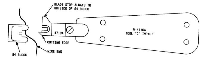
Fig. 5—R-4710A "C" Impact Tool and 94-Type Connecting Block
