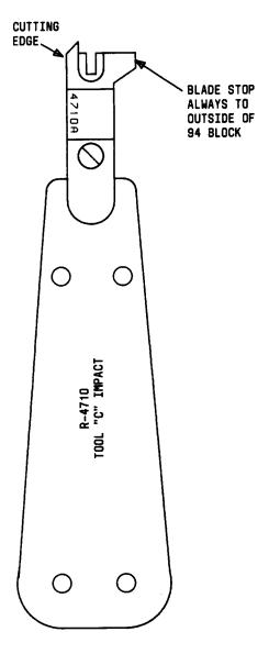
Fig. 1—R-4710 "C" Impact Tool With 4710A Blade
