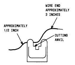
Fig. 4—94-Type Connecting Block With Dressed Conductor
