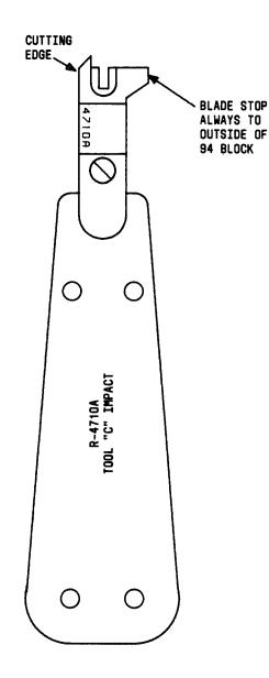
Fig. 2-R-4710A "C" Impact Tool With 4710A Blade
