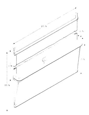
Fig. 1—769A Tool Distributing Frame Bag
