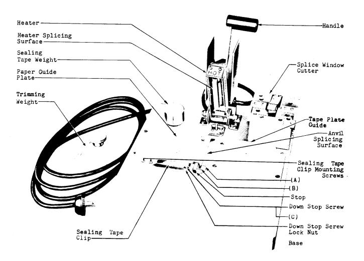
Fig. 2 - Nos. 604B and 604C Splicers
