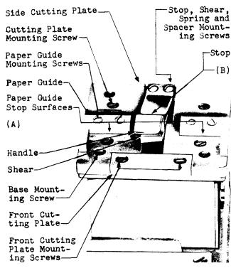
Fig. 5 - Splice Window Cutter (Nos. 604B, 604C, and 604E Splicers)
