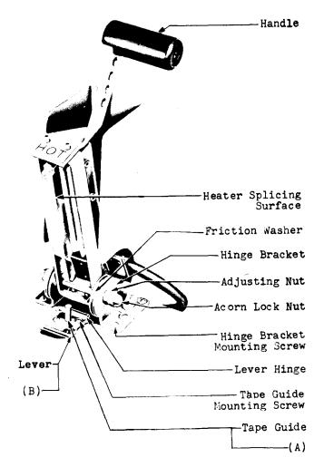
Fig. 4 - Heater and Tape Guide Assembly
