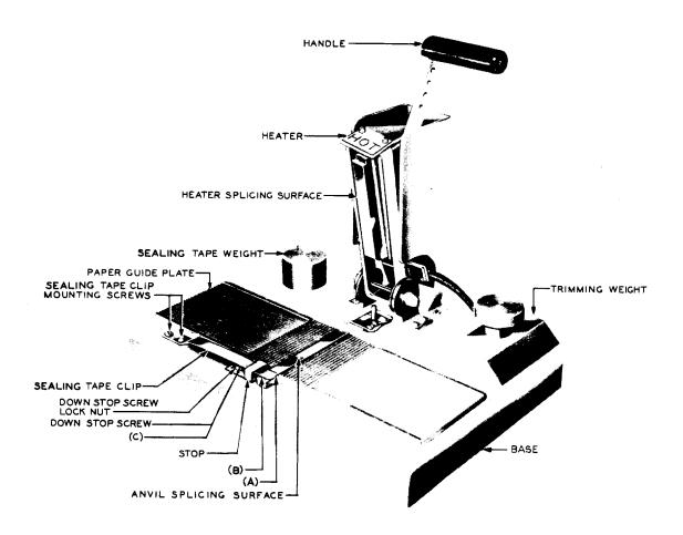
Fig. 1 - Nos. 604A and 604D Splicers (No. 604D Splicer Illustrated)
