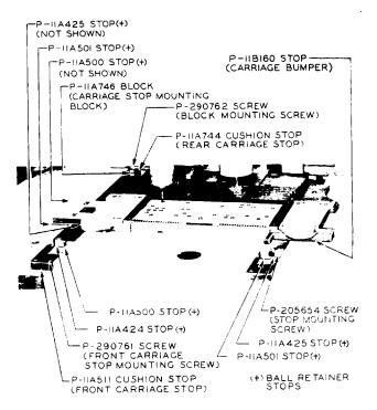
Fig. 13 – Carriage and Ball Retainer Stops and Carriage Bumper
