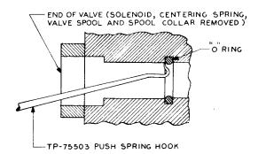
Fig. 24 – Removing "O" Ring From Interior of Valve Having Single Cover
