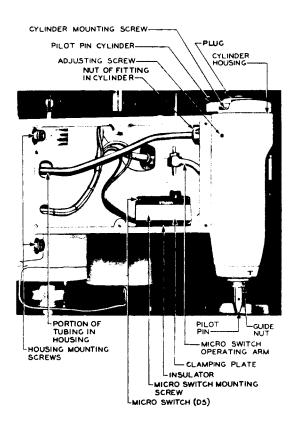
Fig. 25 – Hole-Enlarging Control Unit (cover removed) ---- 659A and 659D Tools Only
