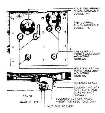
Fig. 19 – Punch and Die Assembly Mounting Details (underside of table)
