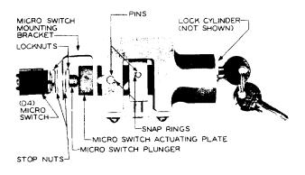
Fig. 31 – Carriage and Power Switch Lock (underside of table)
