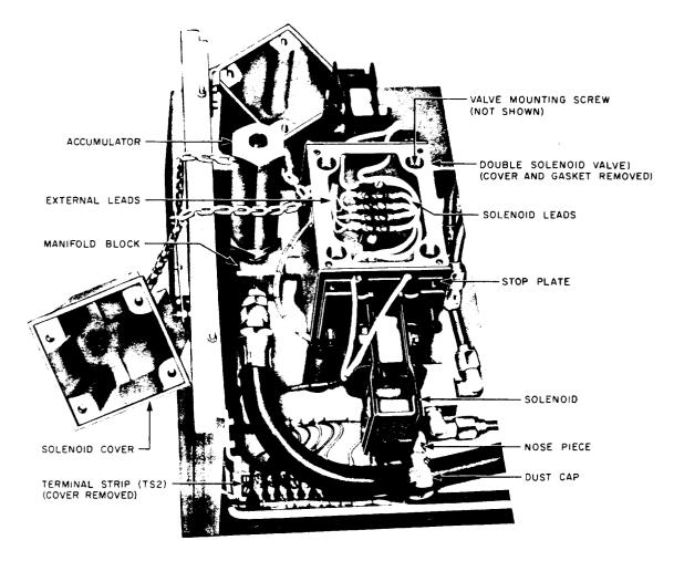
Fig. 23 – Hydraulic Shelf Assembly (partial view with double-solenoid valve cover and gasket removed)
