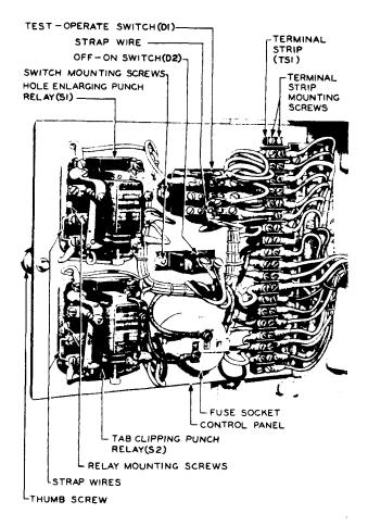
Fig. 33 – Control Panel (open position)
