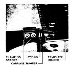
Fig. 28 – Tab-Clipping Control Stylus (elevated position viewed from side)
