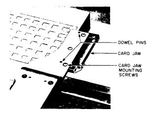
Fig. 30 – Card Nest Jaws With Plate for Supporting Card
