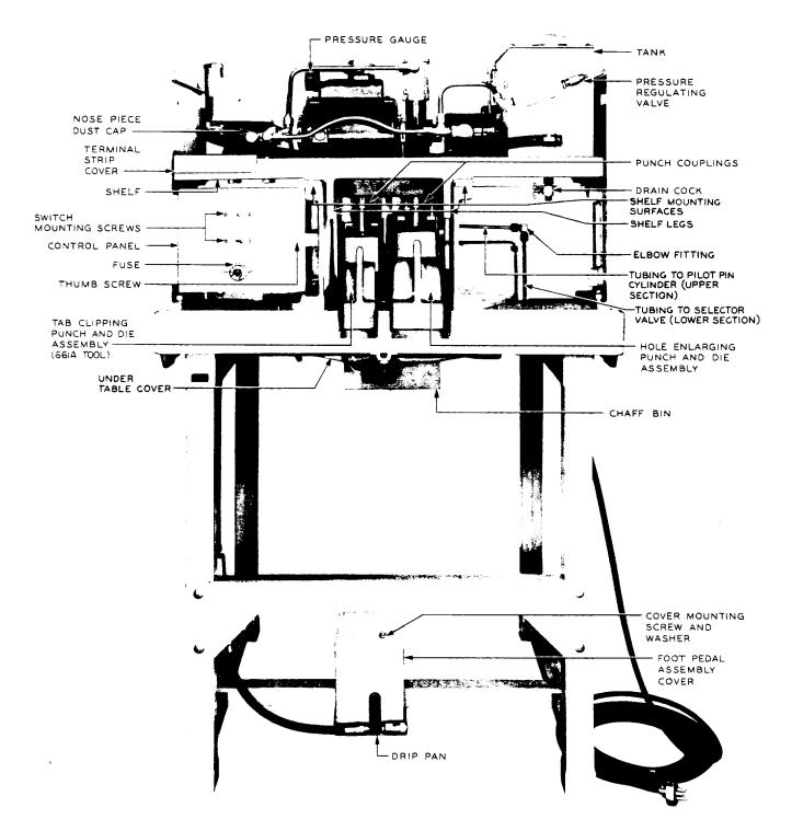
Fig. 17-659A and 659D Tools (rear view - covers removed)
