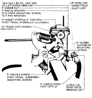
NOTEI:GRC 27-7" O"RING (2 REQ.) (SHAFT "O"RING) GRC 27-9" O"RING (PISTON "O"RING) BELL INDUSTRIES NOTE 2: ALSO ORDER, IF REQUIRED, FEMALE COUPLING, CAT. NO. 846FS-I/4 TUBE X I/8 NPT, IMPERIAL BRASS MANUFACTURING CO. (FOR END OF HOSE NOT SHOWN)
