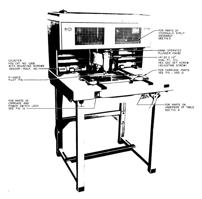
Fig. 2 - 659-Type Tool - 659B, 659C, 659E, and 659F Tools Shown
