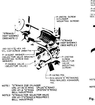
Fig. 10 – Tab-Clipping Control Unit (partial view from below right front of table) — 659A and 659D Tools Only
