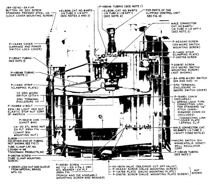
NOTE 1-IF TUBING TO BE REPLACED IS CONNECTED BY BLACK FITTINGS ALSO ORDER FITTINGS TO WHICH EACH END OF TUBING IS CONNECTED. 2-IF FITTING TOBE REPLACED IS BLACK, ORDER TUBING CONNECTED TO FITTING AND ALSO FITTING TO WHICH OTHER END OF TUBING IS CONNECTED.
