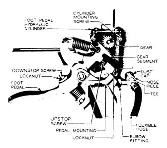
Fig. 29 – Foot-Pedal Assembly (drip pan and covers removed) — 659A and 659D Tools Only
