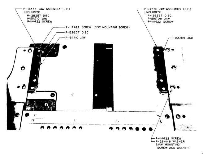
Fig. 14 - Card Nest Jaws With Discs for Supporting Cards
