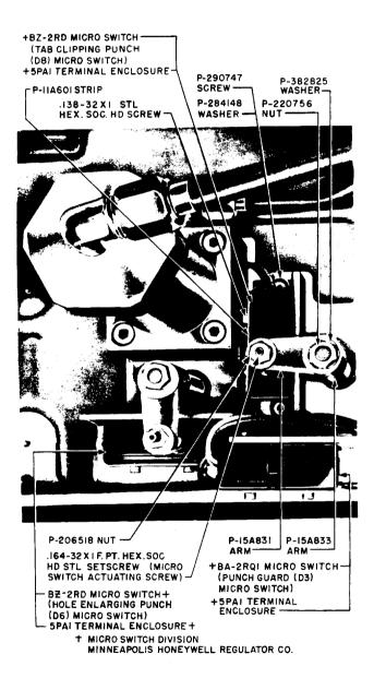
Fig. 8 – Hydraulic Shelf Micro Switches and Associated Parts (viewed from top)
