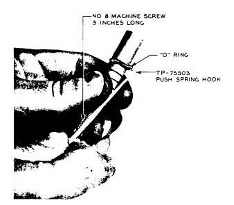
Fig. 26 – Removing "O" Ring From Upper Section of Pilot Pin Shaft — 659A and 659D Tools Only
