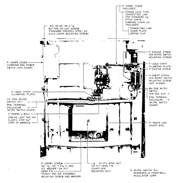
Fig. 4 – 659B, 659C, 659E, and 659F Tools — Underside of Table
