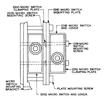
Fig. 32 – Selector-Handle Micro Switches
