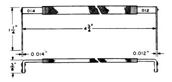
0.012 inch and 0.014 inch Double-end Thickness Gauge.
