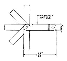
Consists of the 75-type gauges mounted in a handle. The individual gauges are readily removable and replaceable.
