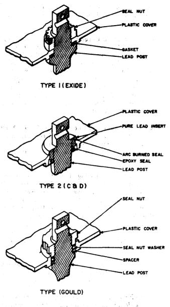
Fig. 11—Battery Post Seals (Typical)
