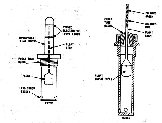
Fig. 2—Rubber Battery Jar Electrolyte Level Indicator Floats
