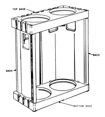
Fig. 6-Basic Module for Four KS-20472 Round Cells
