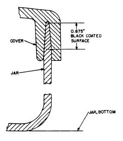
Fig. 2-KS-20472 Round Cell Jar-to-Cover Seal
