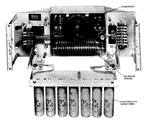
Fig. 3—J86254B, List 1 Rectifier—Rear View—Cover Off
