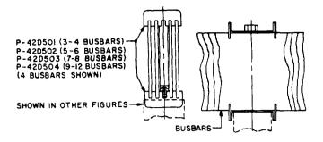
Fig. 3 — Bus-Bar Supports — Three to Twelve Bus Bars
