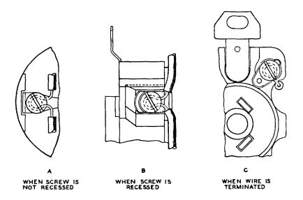
**Note:** The lead should come in at left and continue around clockwise at least 270 degrees to the right but should not cross over itself. An upturned lug or confined space adjacent to the terminal screw plus the looping of the lead should be sufficient to prevent the lead from becoming disconnected if the terminal screw should come loose. Fig. 18 joints need not be soldered unless specified.
