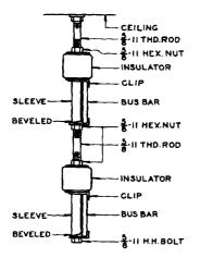
Fig. 7 - Bus-Bar Support from Ceiling-Two Levels
