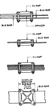
Fig. 10 - Bus-Bar Splice Joints
