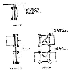
Fig. 13 — Typical Bus-Bar Connections
