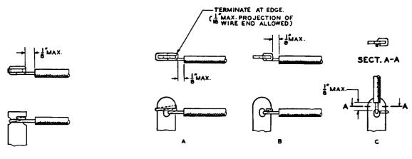
Fig. 14 — Single- or Double-Notched Terminals (double notch shown)
