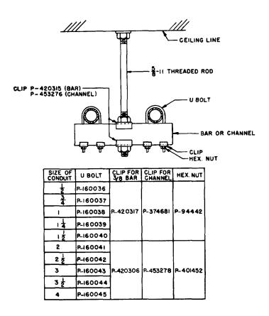
Fig. 25 — Conduit Support for Two Conduits Where Auxiliary Framing Is Not Used
