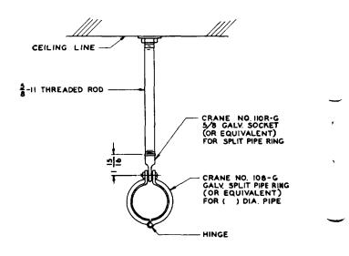
Fig. 24 — Conduit Support for Single Conduit Where Auxiliary Framing is Not Used
