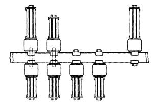
Fig. 9 – Typical Bus-Bar Support Arrangements
