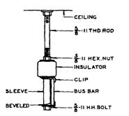
Fig. 6 - Bus-Bar Support from Ceiling-One Bus Bar
