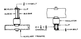
Fig. 1 — Bus-Bar Support — One Bus Bar
