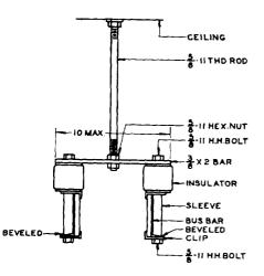
Fig. 8 - Bus-Bar Support from Ceiling-Same Level
