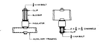
Fig. 2 — Bus-Bar Support — Two Bus Bars
