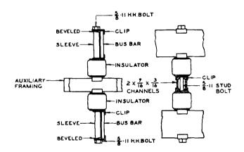
Fig. 4 — Bus-Bar Support — Double-level Bus Bar
