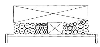
Fig. 20 — Power and Switchboard Cable on Cable Rack—Typical Section
