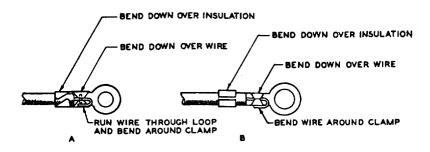
Fig. 16 — Terminals With Two Clamps (F. R. Zierickor H. B. Sherman-type terminal)
