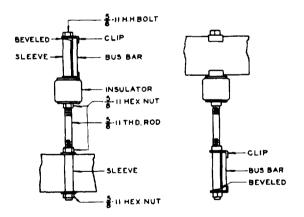
Fig. 5 — Bus-Bar Support — One Bus Bar from Another
