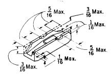
Fig. 2—Maximum Permissible Chips in Spring Groove Walls
