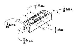
Fig. 3—Maximum Permissible Chips in Moat Walls
