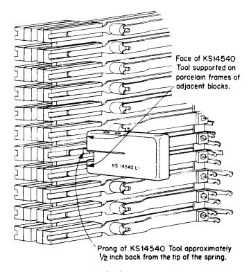
Fig. 1—Method of Using KS-14540 Tool
