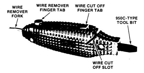
Figure 3. 950C-Type Wire Insertion/Removal/Cutter Tool
