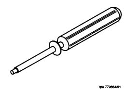
Figure 18. KS-20827, L1 Wire Unwrapping Tool
