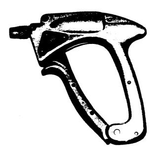
Figure 13. KS-16363, L3 Wire-Wrapping Tool
