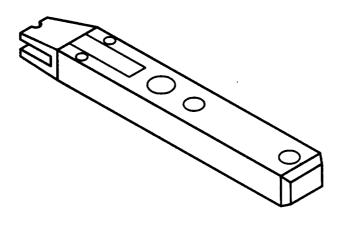
Figure 2. Insertion Bit for 756C-Type Tool
