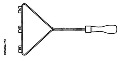
Figure 22. KS-22616, L1 Block Removal Tool
