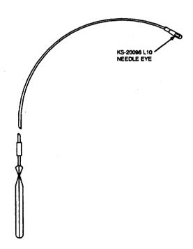
Figure 33. KS-20096, L1 Wiring Needle
