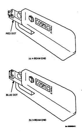
Figure 5. 756C3 Wire Insertion Tool (DA)
