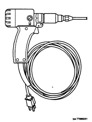
Figure 14. KS-21232, L1 Electric Wire-Wrapping Gun
