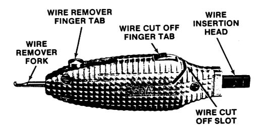
Figure 6. 950A Cutoff/Insertion/Removal Tool (DA)
