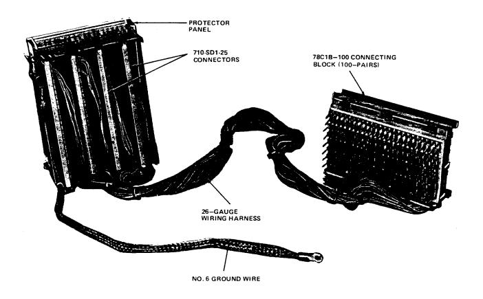
Figure 2. 307A1-100 Connector — Back View
