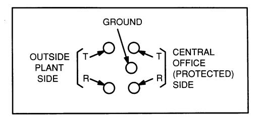
Figure 39. Jack for Protector Unit on 303-, 305-, 307-, 309-, 310-, 310M-, and 311-Type Connectors
