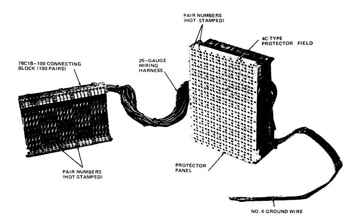
Figure 1. 307A1-100 Connector — Front View
