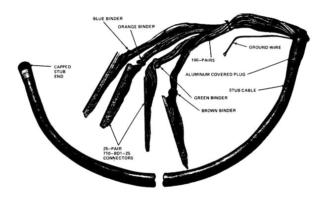
Figure 13. 11-Type Connectorized Stub Cable
