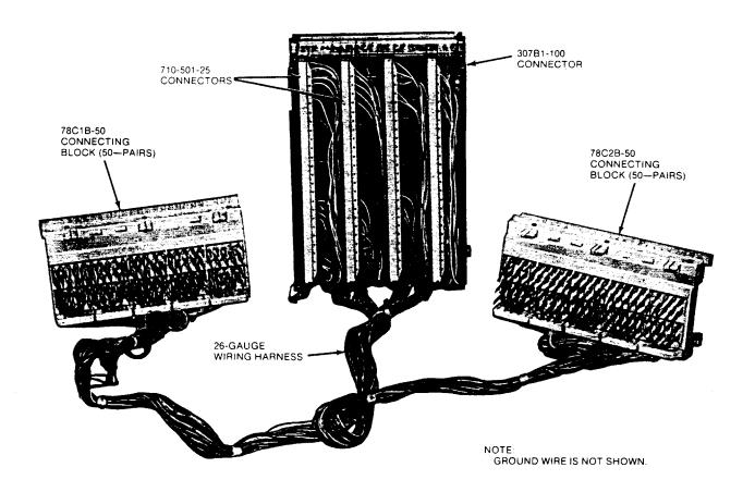
Figure 4. 307B1-100 Connector — Back View
