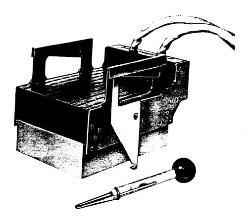
Figure 41. 299B Test Adapter
