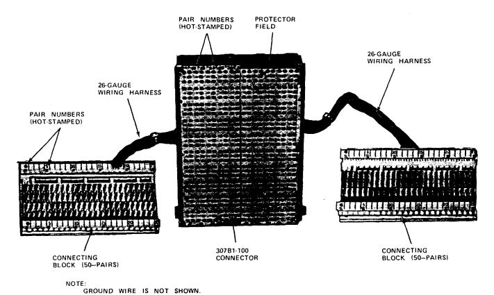
Figure 3. 307B1-100 Connector — Front View
