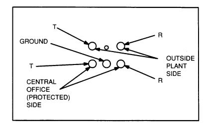
Figure 38. Jack for Protector Unit on 302- and 308-Type Connectors
