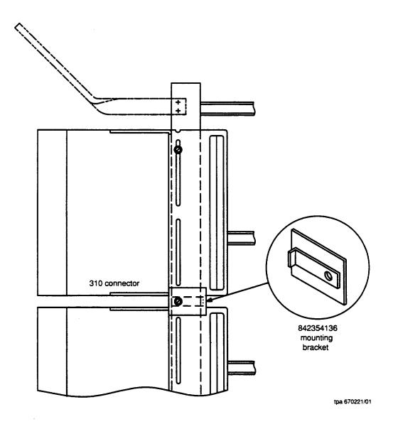
Figure 8. Mounting Arrangement for the 310/310L- or 310M/310ML-Type Connectors at the Top of a Tall Conventional MDF Vertical
