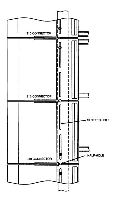
Figure 7. Mounting Arrangement for the 310/310L- or 310M/310ML-Type Connectors Using Existing Mounting Holes
