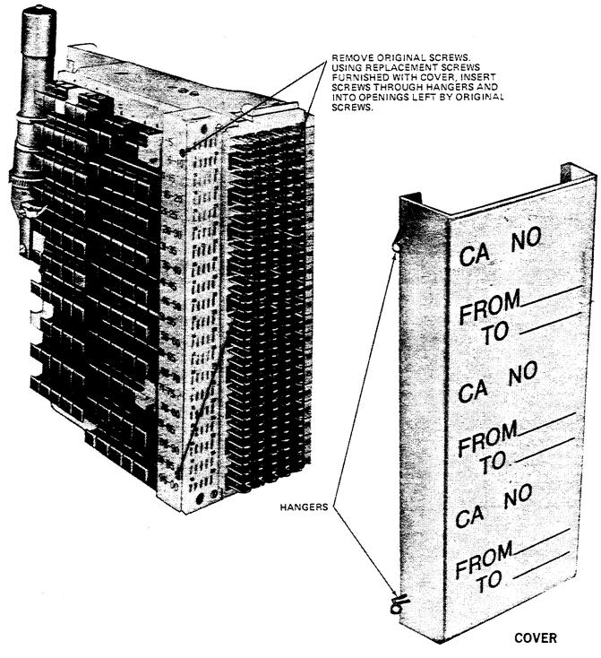
Figure 12. Installing Cover on Connector
