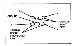
Figure 20. Jack for Protector Unit on 302- and 308-Type Connectors
