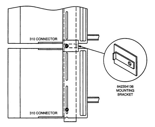
Figure 9. Mounting Arrangement for the 310/310L- or 310M/310ML-Type Connectors at the Bottom of a Tall Conventional MDF Vertical
