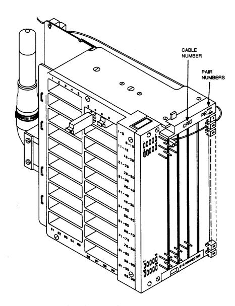
Figure 13. Marking Cable and Pair Numbers
