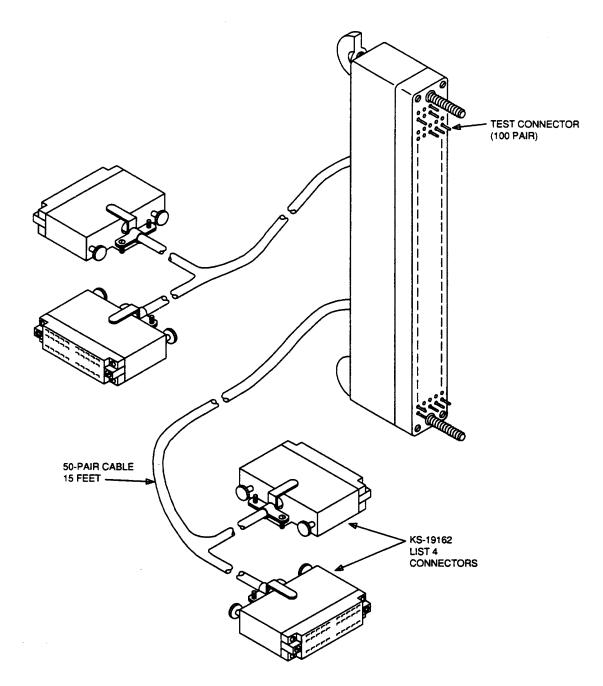
Figure 22. T Test Connector (AT-8987)
