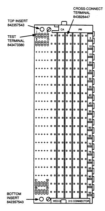
Figure 17. 310-Type Connector, Front View
