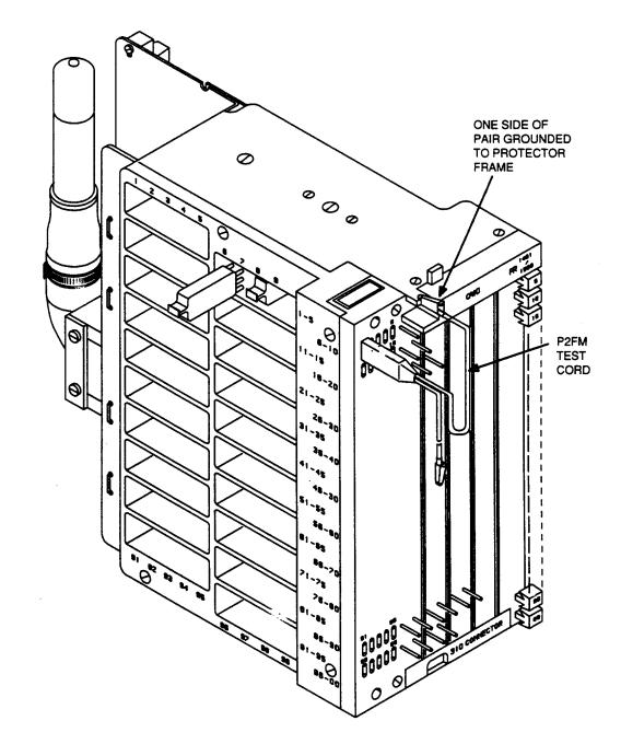
Figure 25. P2FM Test Cord for Testing Individual Pairs
