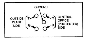
Figure 21. Jack for Protector Unit on 303-, 305-, 307-, 309-, 310-, and 311-Type Connectors
