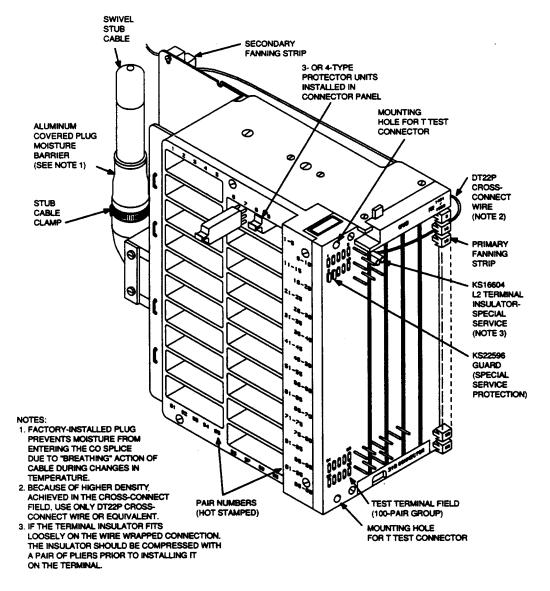
Figure 4. 310-Type Connector — Left Side View — Single Wire-Wrap Cross-Connect Field
