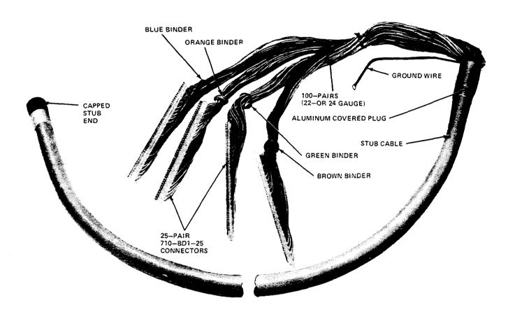
Figure 6. 11-Type Connectorized Stub Cable
