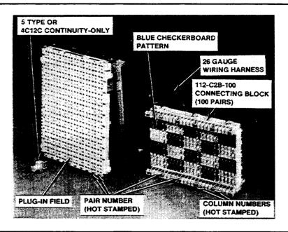
Figure 2. 407D1-100 Connector — Front View
