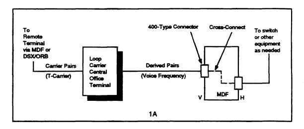
Figure 1. Typical Application with Digital Loop Carrier Systems (Sheet 1 of 2)
