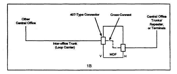
Figure 1. Typical Application with Digital Loop Carrier Systems (Sheet 2 of 2)
