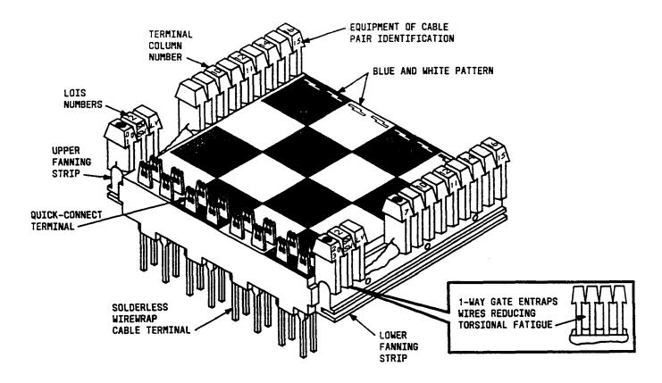
Figure 10—112-Type Connecting Block Features
