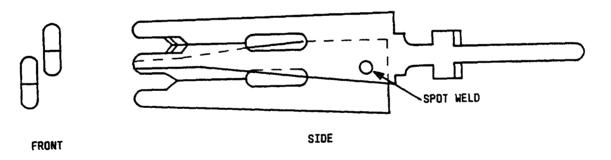
Figure 5—Views of Terminal Used on 78C-Type Connecting Blocks
