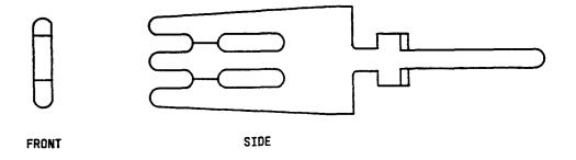
Figure 11—Views of Quick-Clip Terminal Used on 112-Type Connecting Block
