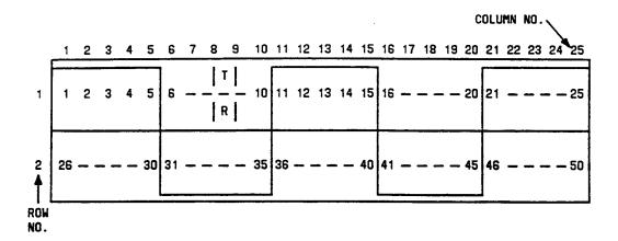
Figure 6—Typical 50-Pair Terminal Arrangement (Example is 78C1A-50)
