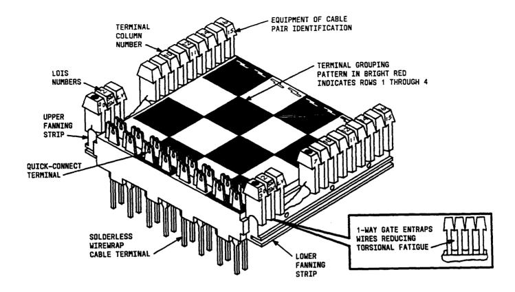
Figure 4—78C-Type Connecting Block Features
