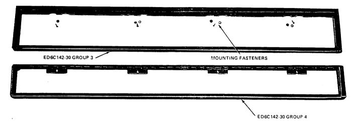
Figure 18—112H Series Connecting Block Mounting Adapters
