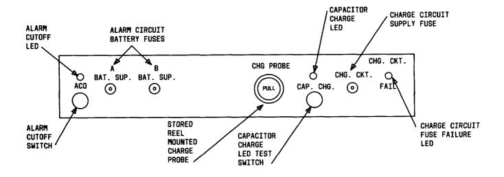
Fig. 3—Control Panel Assembly
