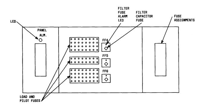
Fig. 2—Filter-Fuse Panel Assembly
