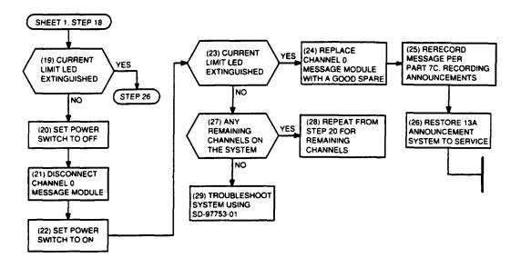
Figure 9. Current Limit LED (Sheet 2 of 2)
