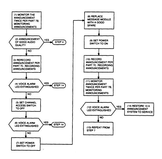
Figure 12. Voice Alarm LED—Message Modules Series 15 or Higher and UD7 Message Module
