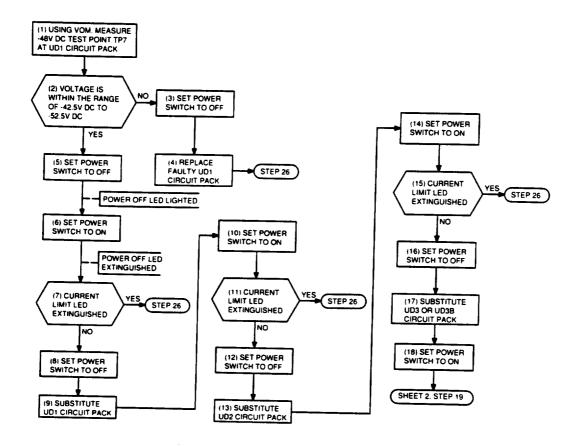
Figure 9. Current Limit LED (Sheet 1 of 2)
