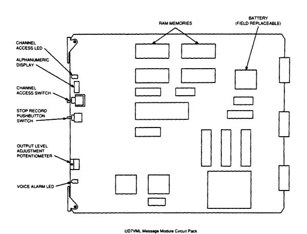
Figure 6. UD7 VML Message Module Circuit Pack
