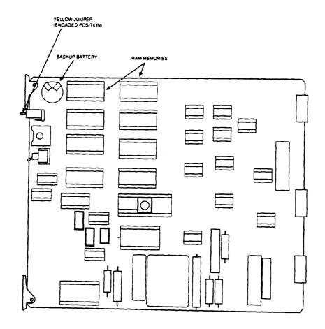
Figure 5. UD4 VML Message Module Circuit Pack (Series 15 or Higher) With RAM Memories
