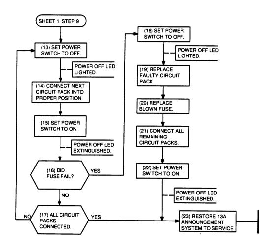
Figure 8. Blown Fuse (Sheet 2 of 2)
