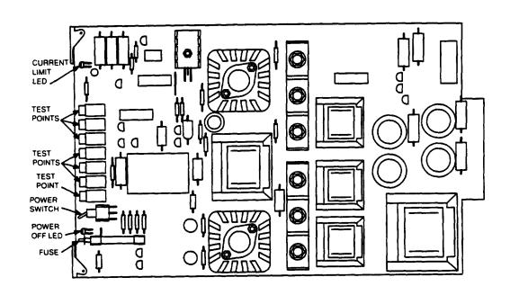
Figure 2. UD1/UD8 Power Supply Circuit Pack
