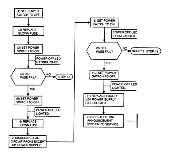
Figure 8. Blown Fuse (Sheet 1 of 2)
