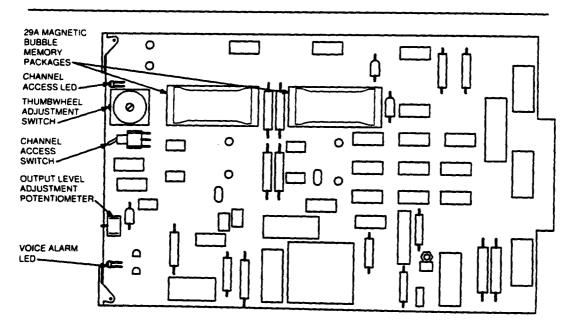
Figure 4. UD4 VML Message Module Circuit Pack (Series 1 Through 14) With 29A Bubble Memories
