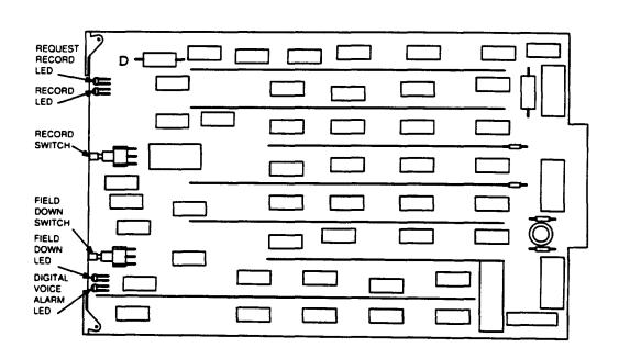
Figure 3. UD3B Timing and Control Circuit Pack
