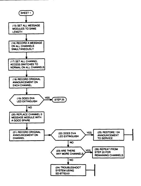
Figure 11. Digital Voice Alarm LED—Message Modules Series 1 Through 14 Only (Sheet 2 of 2)
