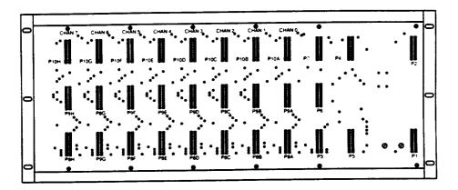
Figure 7. 13A Printed Wiring Backplane
