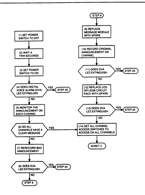
Figure 11. Digital Voice Alarm LED—Message Modules Series 1 Through 14 Only (Sheet 1 of 2)
