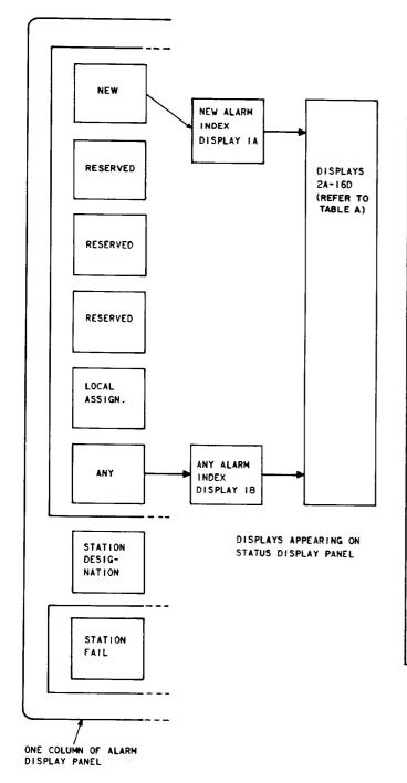
Fig. 6—Alarm Display for Stations Having More Than Four Status Displays (New Assignment Philosophy)
