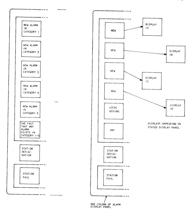
Fig. 4—Alarm Display—Typical Indicator Assignment
