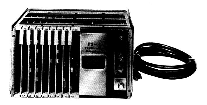
Fig. 1—Telemetry-to-Computer Translator (TCT)
