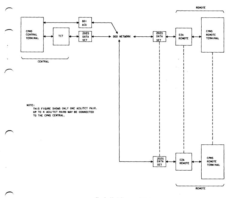
Fig. 3-Block Diagram of CPMS
