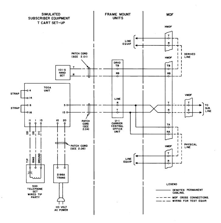
Fig. 1—Central Office U1 Carrier Test Arrangement
