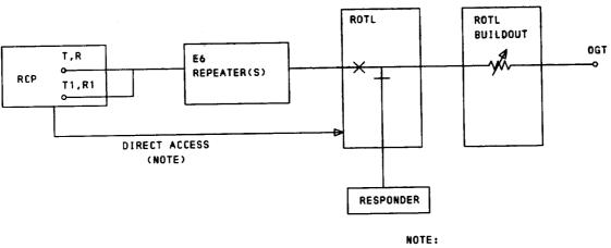
THE DIRECT ACCESS OPTION MUST BE PROVIDED IN THE ROTL FRAME Í
