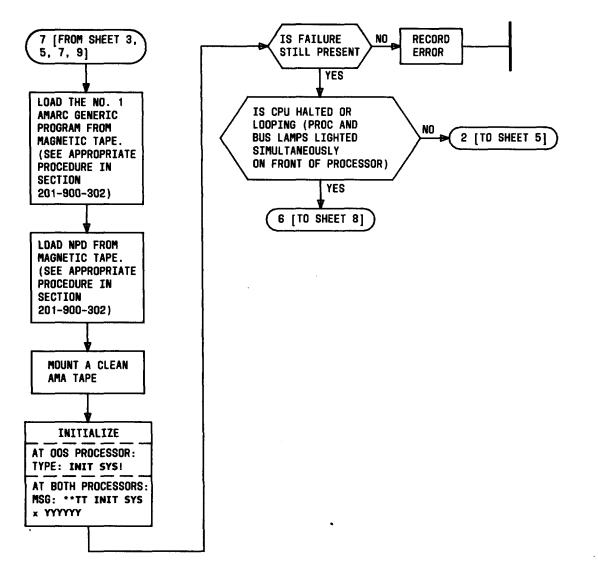
Fig. 2—Fault Isolation Procedure Flow Diagram (Sheet 4 of 10)4
