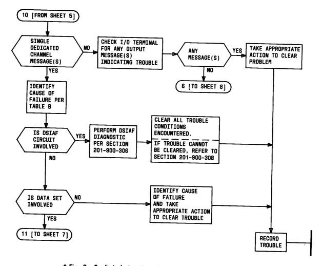
♦ Fig. 2—Fault Isolation Procedure Flow Diagram (Sheet 6 of 10)♦
