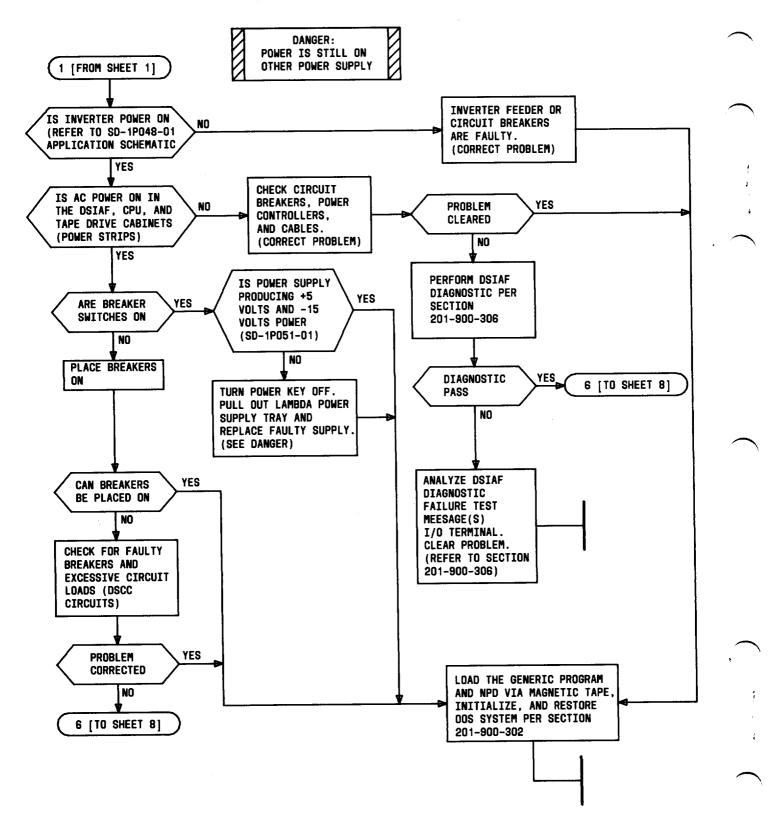
♦ Fig. 2—Fault Isolation Procedure Flow Diagram (Sheet 10 of 10)♦
