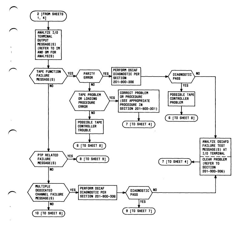
Fig. 2—Fault Isolation Procedure Flow Diagram (Sheet 5 of 10)\$
