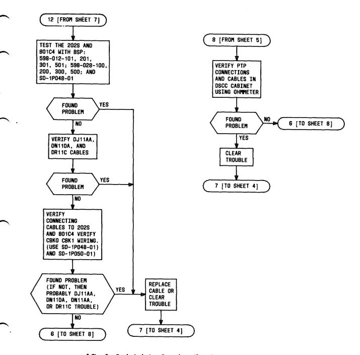
♦ Fig. 2—Fault Isolation Procedure Flow Diagram (Sheet 9 of 10)
