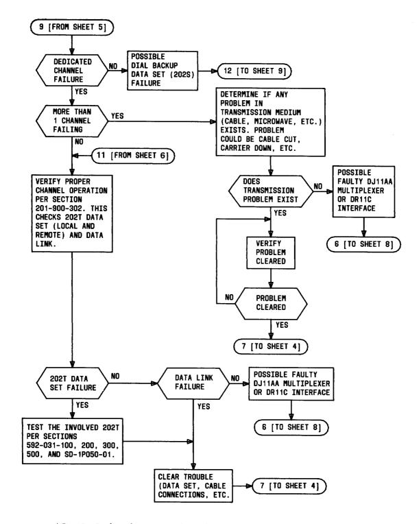
♦ Fig. 2—Fault Isolation Procedure Flow Diagram (Sheet 7 of 10) ♦
