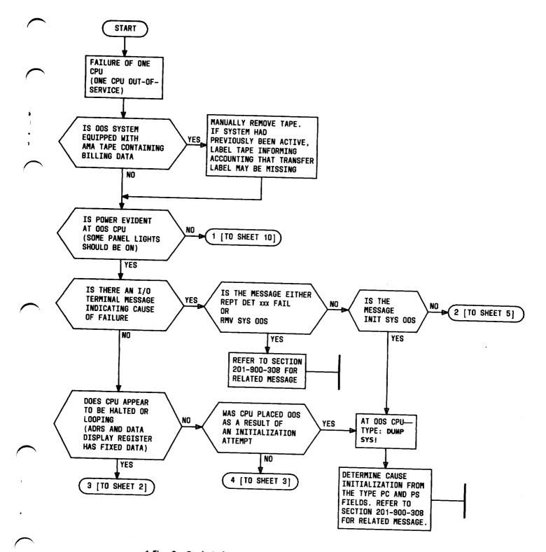
♦ Fig. 2—Fault Isolation Procedure Flow Diagram (Sheet 1 of 10)♦
