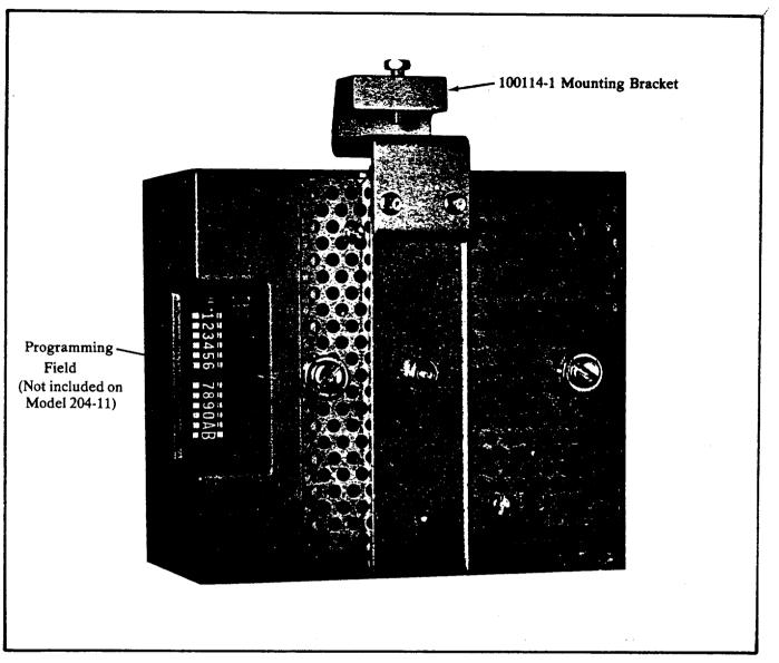
Figure 6. TonePulse Converter (Rear view)
