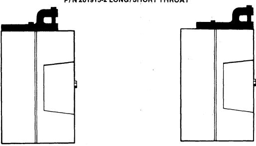
A typical mounting behind a linefinder is shown here. This configuration is used where there are no wires, components or other protrusions extending beyond the channel. This mounting configuration is used when components or other protrusions occur up to 0.75 inches beyond the channel.
