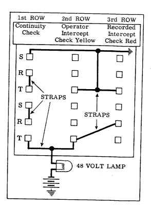
Figure 4 — Test Circuit for Intercepting Connectors INSTALL ON SPARE LUGS
