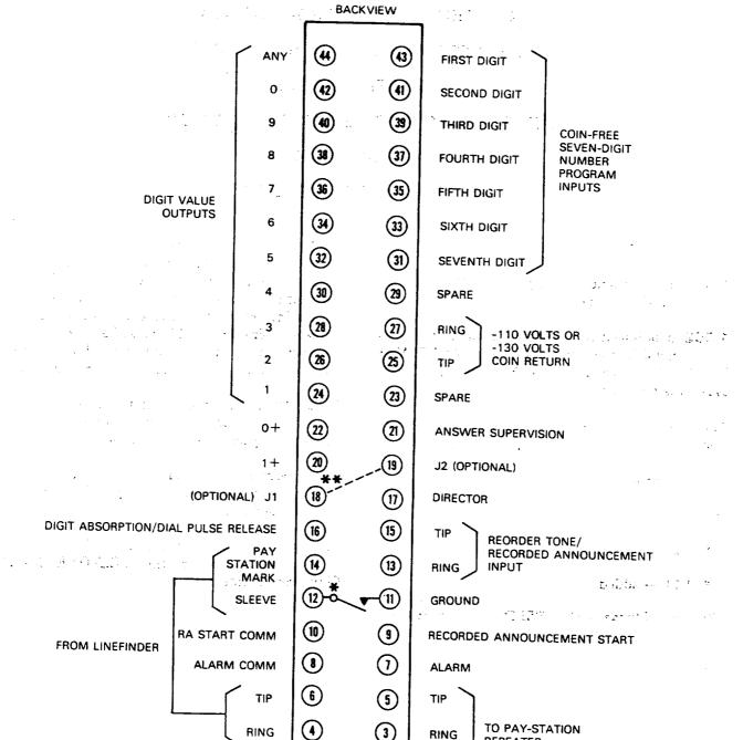
\* Pins 11 and 12 short together to automatically busy out the linefinder when the circuit card is not inserted into the connector.
