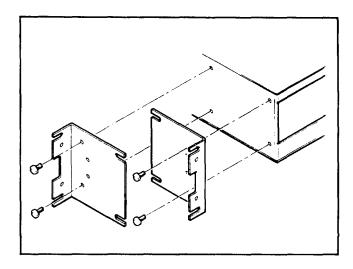
Fig. 3 Bracket Attachment 19 in. Rack Mounting
