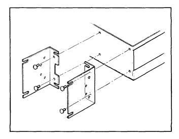
Fig. 4 Bracket Attachment 23 in. Rack Mounting
