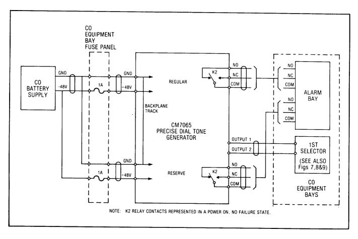
Fig. 6 Typical Connections
