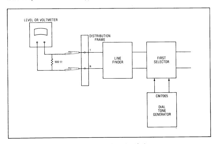
Fig. 12 Test Connections --- Level Setting
