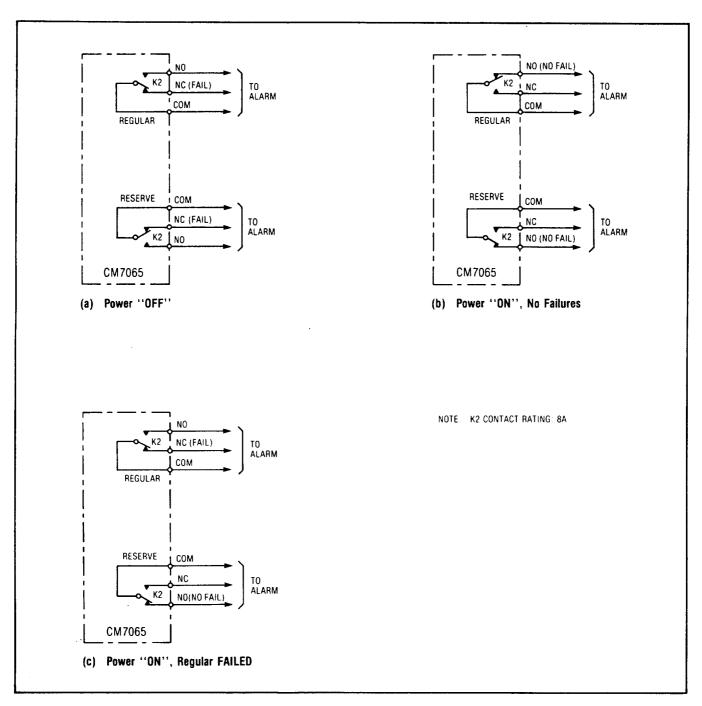
Fig. 10 Alarm Relay States
