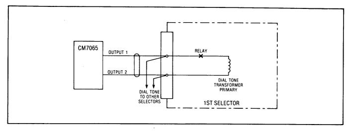
Fig. 7 1st Selector Connections: Western Electric
