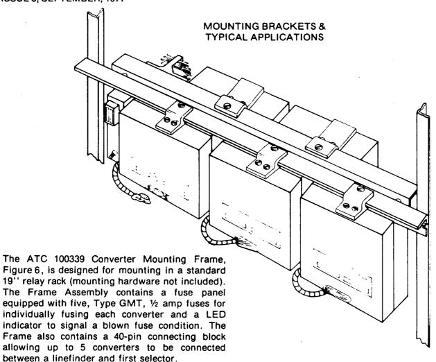
FIGURE 6 100339 MOUNTING FRAME ASSEMBLY
