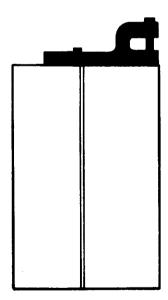
This configuration of side mounting allows 10 converters to fit in the same space as would 9 converters mounted in upright position. The converter in this position has a width of 4.1 inches as opposed to 4.7 inches when mounted in the upright position.
