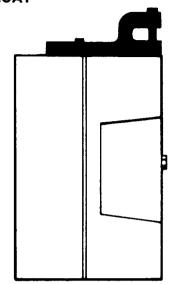
A typical mounting behind a linefinder is shown here. This configuration is used where there are no wires, components or other protrusions extending beyond the channel. This mounting configuration is used when components or other protrusions occur up to 0.75 inches beyond the channel.
