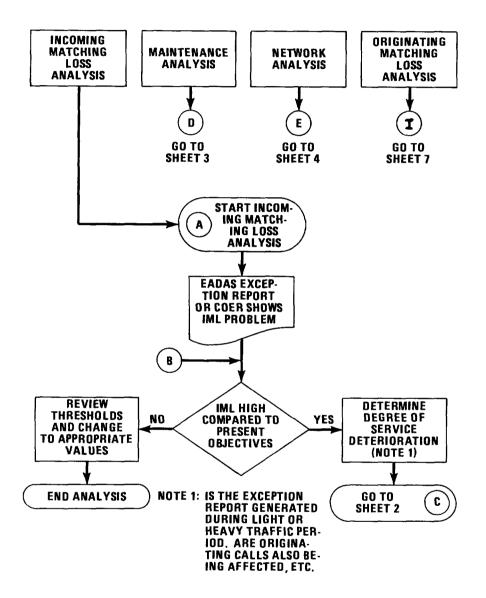
Figure 1 - Analysis Flowchart (Sheet 1 of 8) (10.01, 10.02)
