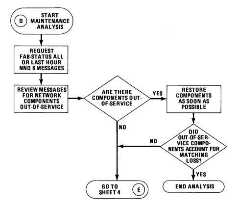
Figure 1 - Analysis Flowchart (Sheet 3 of 8) (10.01, 10.02, 10.06)
