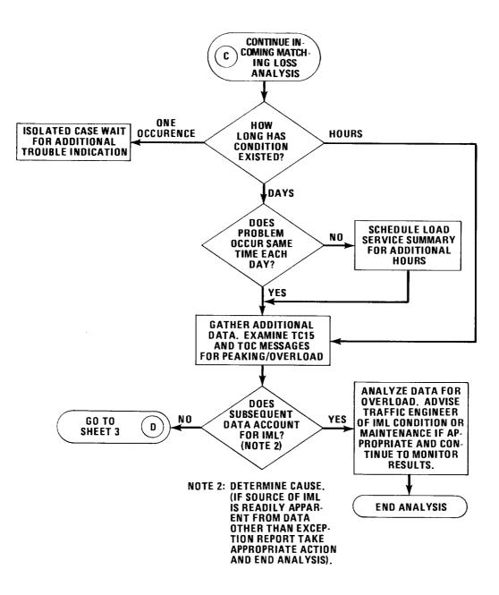
Figure 1 - Analysis Flowchart (Sheet 2 of 8) (10.01, 10.02)
