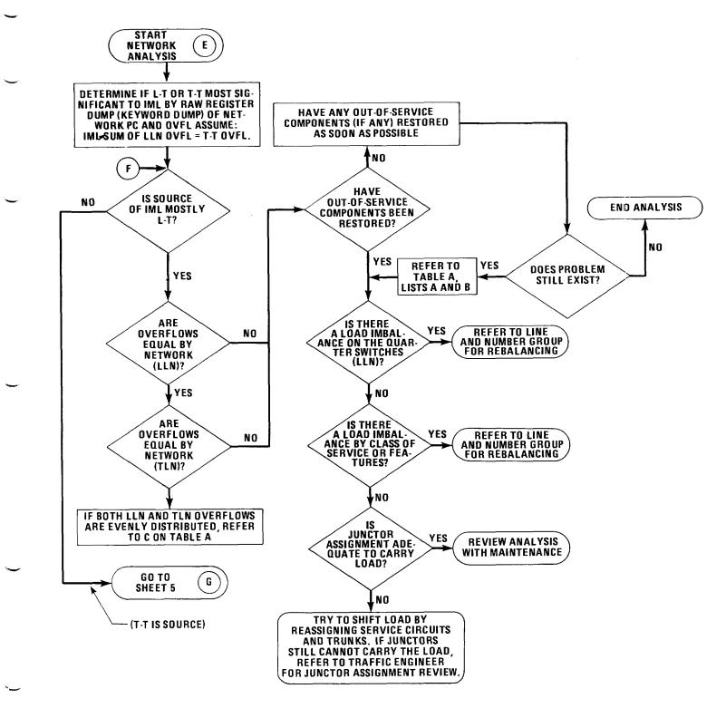
Figure 1 - Analysis Flowchart (Sheet 4 of 8) (10.01, 10.02, 10.03)
