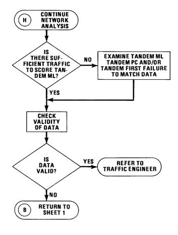
Figure 1 - Analysis Flowchart (Sheet 6 of 8) (10.01, 10.02, 10.03)
