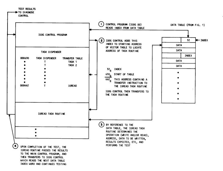
Fig. 2—Table-Driven Diagnostic Test Structure
