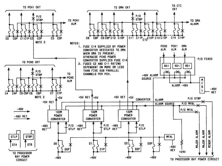
Fig. 12—CTI/Power Unit—Power and Power Alarms
