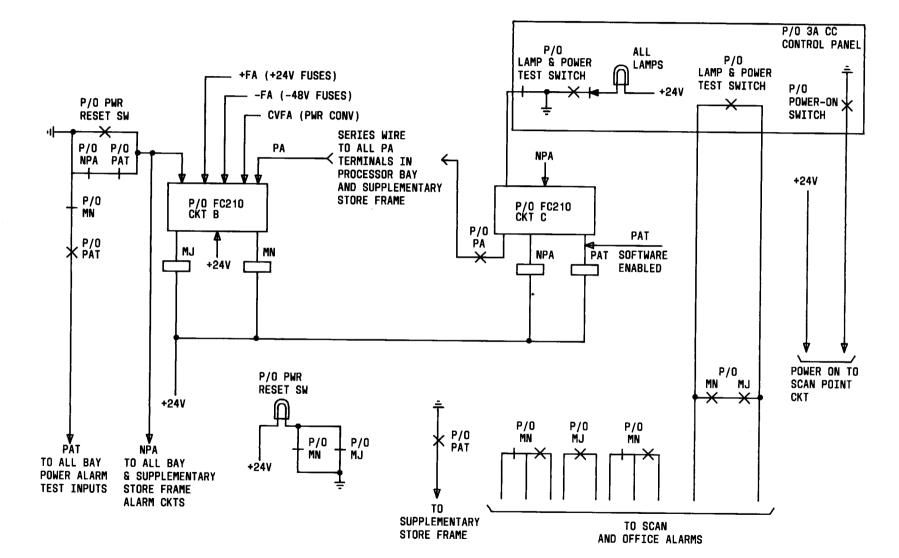
Fig. 9—Processor Frame Power Circuit—Power and Power Alarm Test
