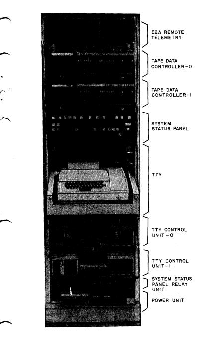
Fig. 3—Common Systems Maintenance Frame
