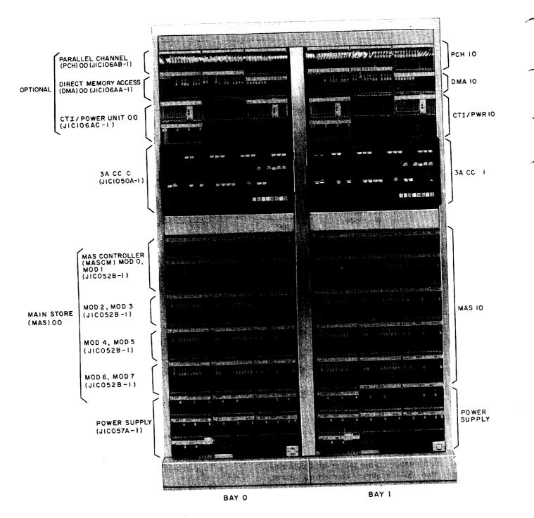
Fig. 2—Typical Processor Frame
