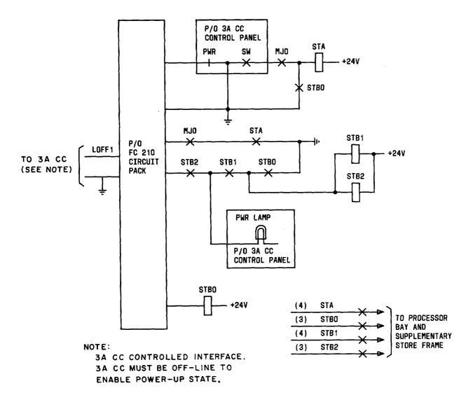
Fig. 8-Processor Frame-Bay Power Control
