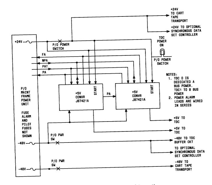
Fig. 16—Tape Data Controller Power and Power Alarms
