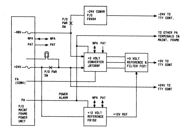
Fig. 17—TTY Controller Unit Power and Power Alarms
