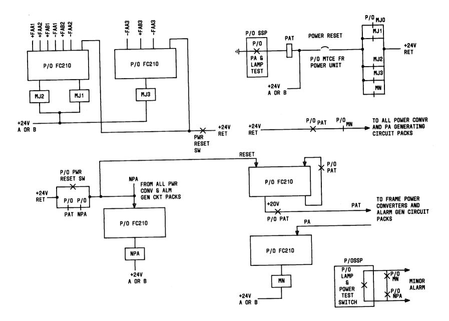
Fig. 15—Maintenance Frame Power Unit—Power Alarm Test and Reset
