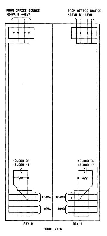
Fig. 6—Typical 3A Processor Frame—Power Input and Filter
