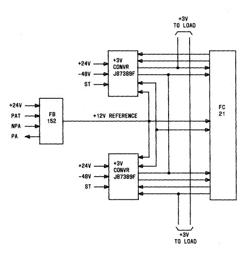
Fig. 10—Typical FC21 Circuit Pack Application
