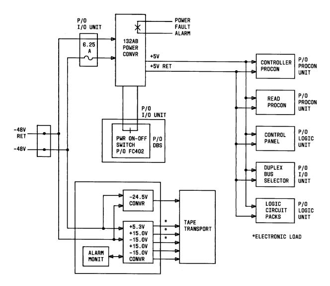
Fig. 18—Programmed Magnetic Tape System Frame—Power Block Diagram
