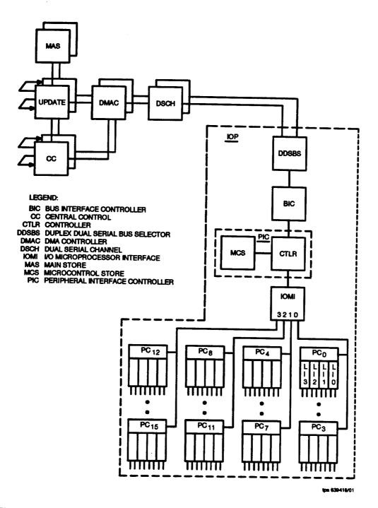
Figure 13. Input/Output Processor Block Diagram
