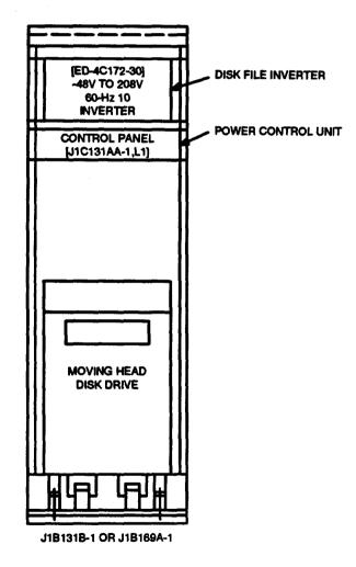
Figure 4. Moving Head Disk Frame (80/300 Mbyte)
