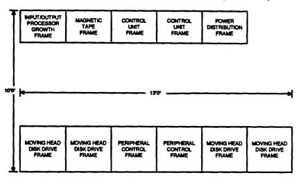
Figure 7. Typical 3B20D Model 1 Computer Floor Plan
