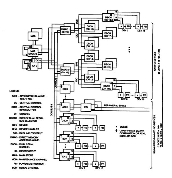
Figure 11. Control Unit Internal Architecture
