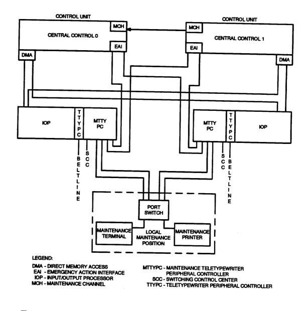
Figure 15. 3B20D Model 1 Computer Maintenance Interfaces
