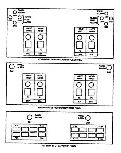
Figure 21. High-Current Fuse Panels
