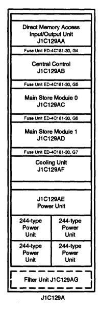
Figure 1. Control Unit Frame
