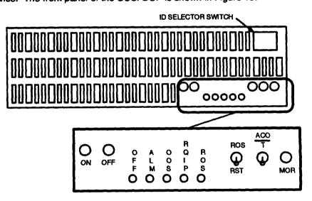
Figure 19. SCSI Disk Unit Package
