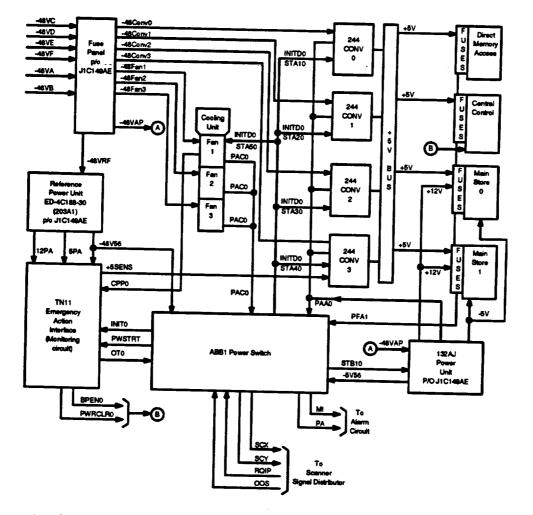
Figure 24. Control Unit Power Block Diagram
