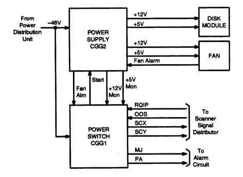
Figure 30. Disk Unit Package Power Block Diagram
