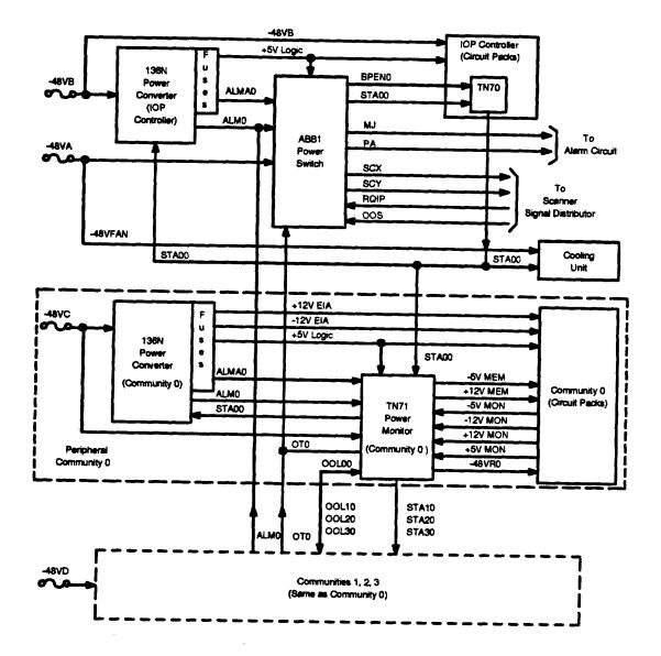
Figure 25. Input/Output Processor Power Block Diagram
