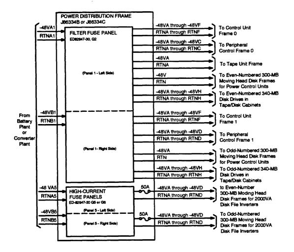
Figure 22. Power Distribution Frame Block Diagram
