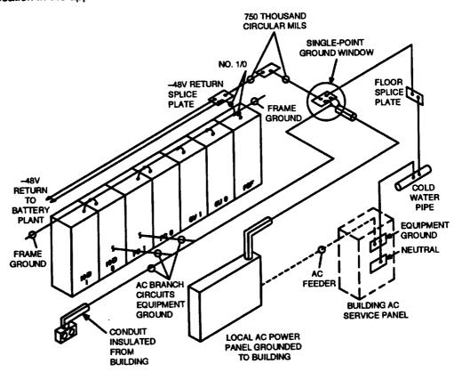
Figure 8. Typical Overhead Single-Point Ground System
