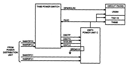
Figure 29. SCSI Disk File Controller Power Distribution
