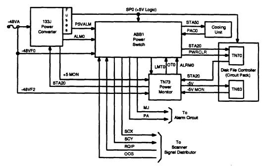
Figure 26. Disk File Controller Power Block Diagram
