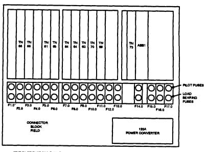
THE PILOT FUSE FOR FUSE F1. IS F1.1. OTHER PILOT FUSES FOLLOW THE SAME NUMBERING CONVENTION.
