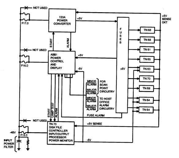
Figure 13. Disk File Controller Unit Power and Alarm Circuit (Generic 2)
