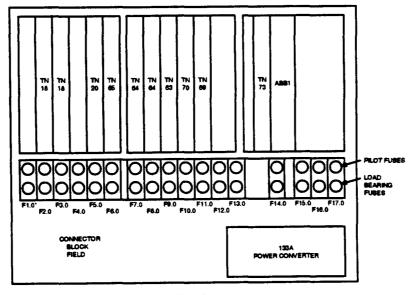
"THE PILOT FUSE FOR FUSE F1.0 IS F1.1. OTHER PILOT FUSES FOLLOW THE SAME NUMBERING CONVENTION.
