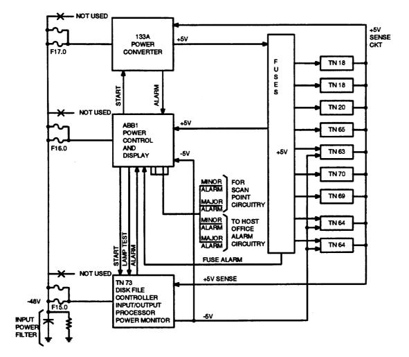
Figure 14. Disk File Controller Unit Power and Alarm Circuit (Generic 3)
