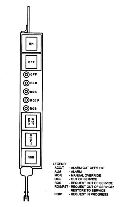
Figure 15. ABB1 Front Panel
