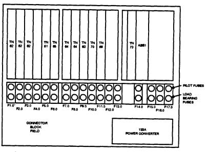
"THE PILOT FUSE FOR FUSE F1.0 IS F1.1 OTHER PILOT FUSES FOLLOW THE SAME NUMBERING CONVENTION.
