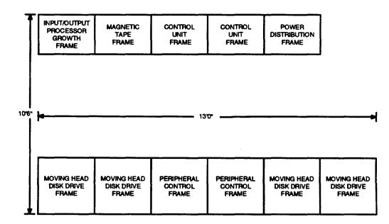
Figure 1. Typical Computer Floor Plan
