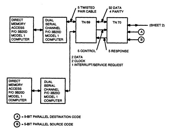
Figure 8. Disk File Controller Unit Block Diagram (Generic 1) (Sheet 1 of 2)
