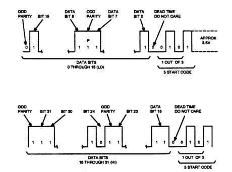
Figure 11. Disk File Controller-Direct Memory Access Message Format
