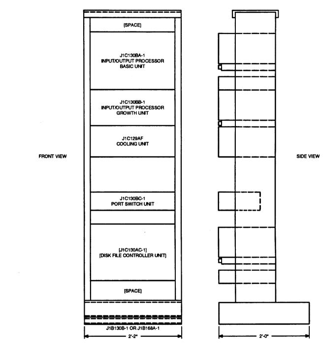
Figure 2. Typical Peripheral Control Frame With Disk File Controller
