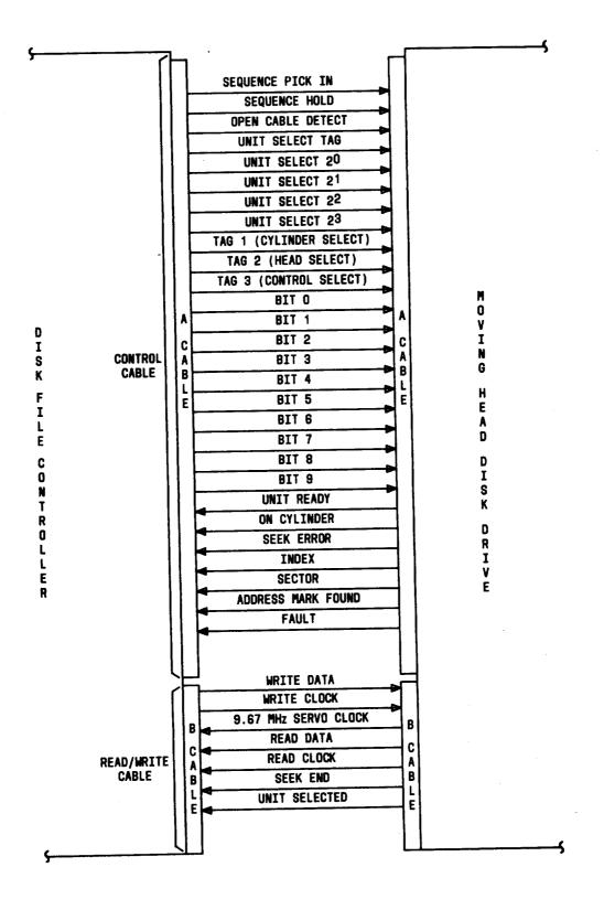
Fig. 7—Control and Read/Write Cables
