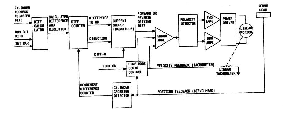
Fig. 10—Basic Servo Block Diagram
