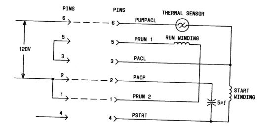
Fig. 14—Pump Motor Wiring Diagram
