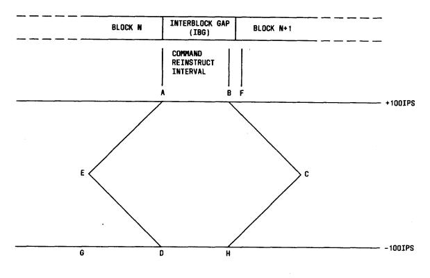
Fig. 17—Streaming Mode Velocity Diagram
