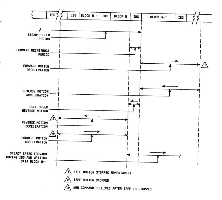
Fig. 22—Tape Motion Control (Receiving Command Following Repositioning Cycle)
