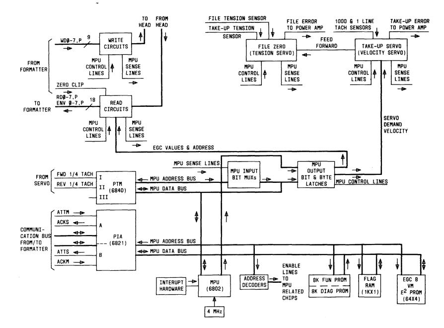
Fig. 9—Read/Write Servo Block Diagram
