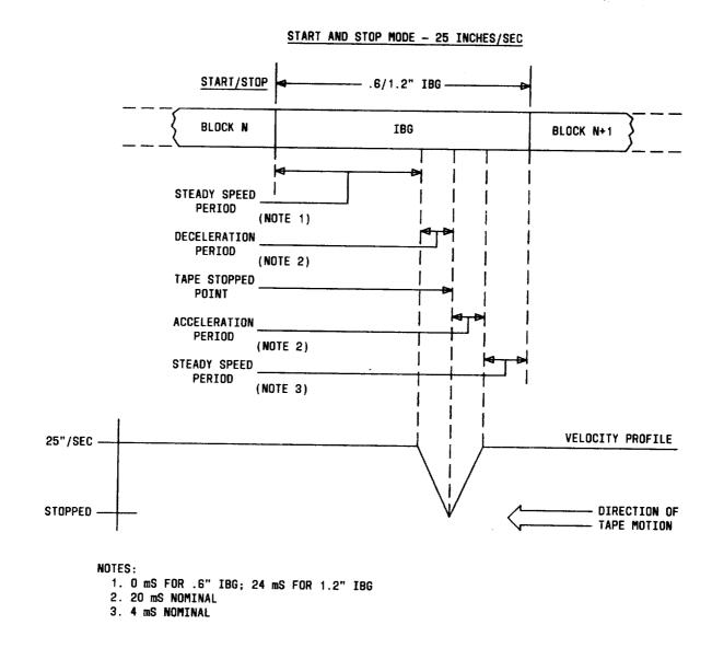
Fig. 16—Start/Stop Mode Tape Motion Control
