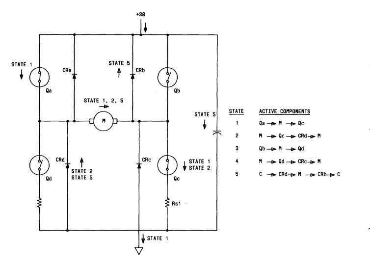
Fig. 12—Bridge Circuit
