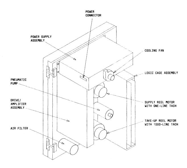
Fig. 6—Tape Deck (Rear View)
