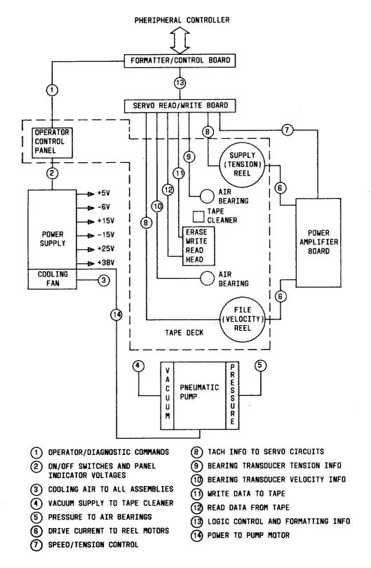
Fig. 7—Tape Unit Functional Block Diagram
