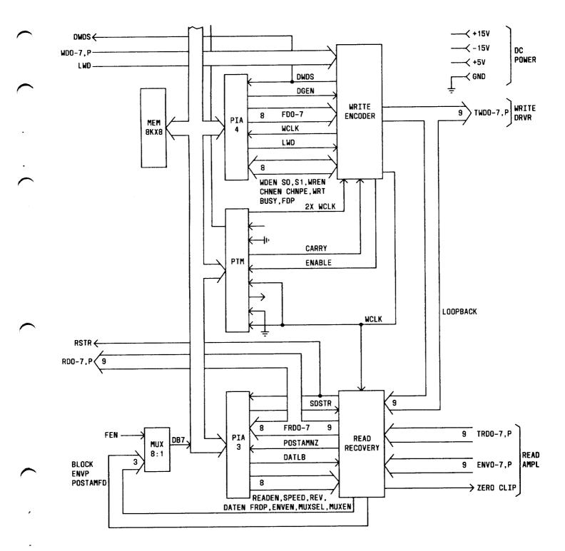
Fig. 8—Formatter/Control Block Diagram (Sheet 2 of 2)
