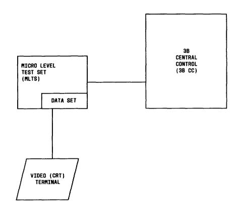
Fig. 3-Micro Level Test Set (MLTS) Application
