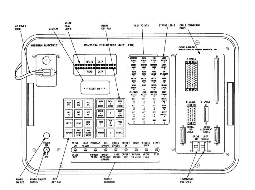
Fig. 5—Field Test Unit
