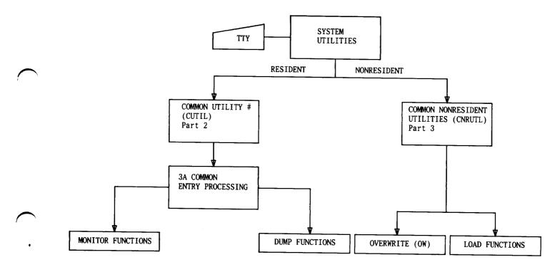
Fig. 2—System Utility Structure
