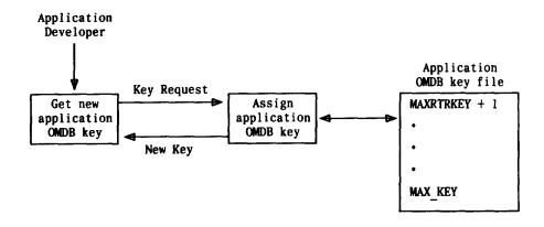
Fig. 11—Application OMDB Key Assignment
