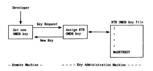
Fig. 10-UNIX RTR OMDB Key Assignment
