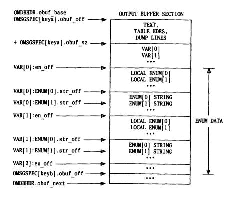
Fig. 7—Layout of Output Buffer Section
