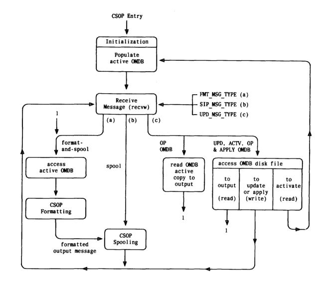
Fig. 12—CSOP High Level Design with OMDB
