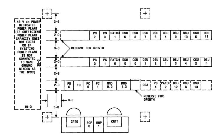
EQUIPMENT 1PSS <u>3B2OD FRAMES</u> MMD - MINI MODULE DISK (0,1,2,3) PC - PROCESSOR CONTROL (0,1) TU - TAPE UNIT CRT - CATHODE-RAY TUBE (0,1) ROP - RECEIVE-ONLY PRINTER <u>OTHER FRAMES</u> CSU - CHANNEL SERVICE UNIT DSU - DATA SERVICE UNIT PD - POWER DISTRIBUTION DSA - DATA SET AND ALARM PATCH - PATCH PS - PACKET SWITCH
