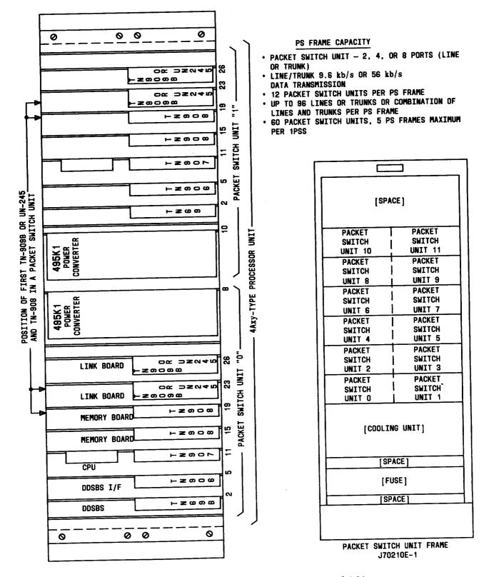
Fig. 4—Packet Switch Frame—Paragraphs 3.02 and 4.06
