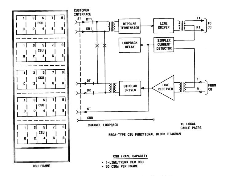
Fig. 7—Channel Service Unit Frame—Paragraphs 3.06 and 4.12
