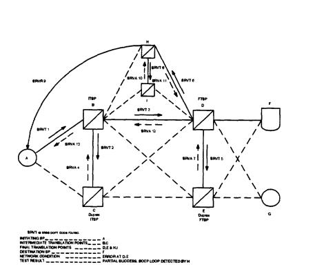
Figure 6-13. Detection of SCCP Routing Loop
