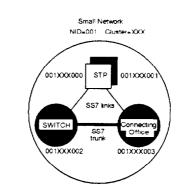
Figure 3-8. Switch Routing Values for Local Scenario
