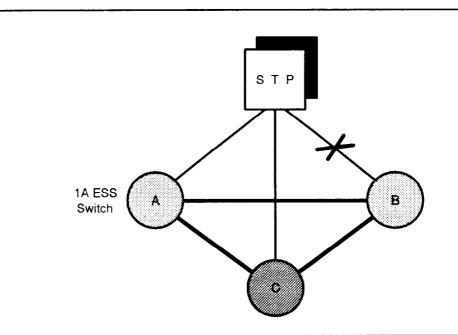
Figure 2-2. Direct Trunks Between End Offices with Overflow to a Local Tandem
