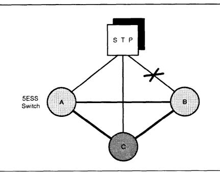
Figure 2-5. Direct Trunks to an End Office with Overflow to Another Tandem
