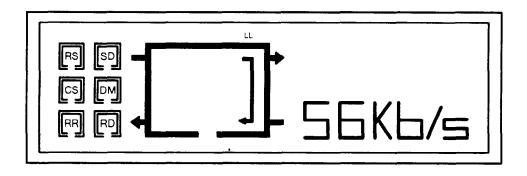
Figure 4-4. Front Display of the Lucent Technologies 2556 DSU With Local Loopback
