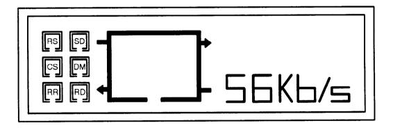
Figure 4-3. Front Display of the Lucent Technologies 2556 DSU Under Normal Operation
