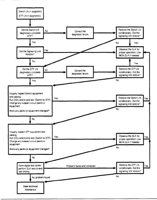
Figure 4-2. Recovery from Declared Link Failure
