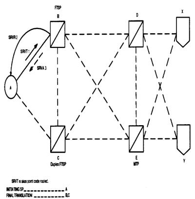
FINAL TRANSLATION \_\_\_\_\_\_ B,C SCCP GT DESTINATION \_\_\_\_\_ Y NETWORK CONDITION \_\_\_\_\_ NO TRANSLATION AT B TEST RESULT \_\_\_\_\_ FAILURE. LOCATION OF ERROR IDENTIFIED.
