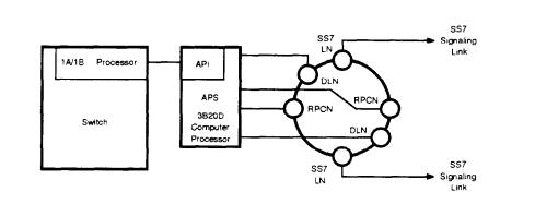
Figure 4-9. Application Processor System
