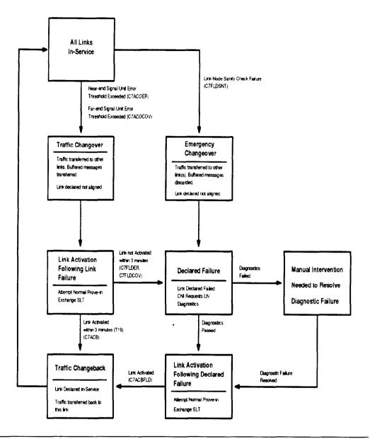
Figure 4-1. Signaling Link Failure Reports
