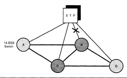
Figure 2-3. Direct Trunks to a Local Tandem with Overflow to Another Local Tandem
