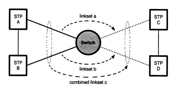
Figure 7-1. Rehoming Switch from One STP Mated Pair to Another
