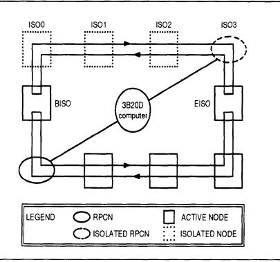
Figure 4-8. A Multiple Node Isolated Ring Segment
