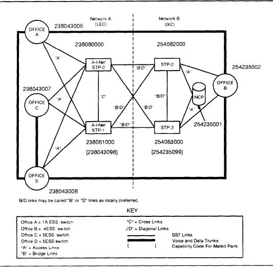
Figure 3-6. Sample LEC Network Interconnect Configuration
