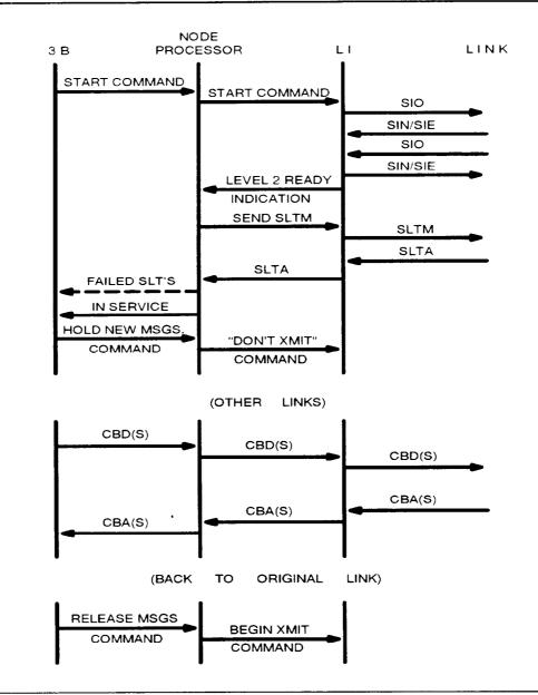
Figure 2-6. Signaling Link Activation
