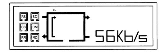
Figure 4-5. Front Display of the Lucent Technologies 2556 DSU with Digital Loopback
