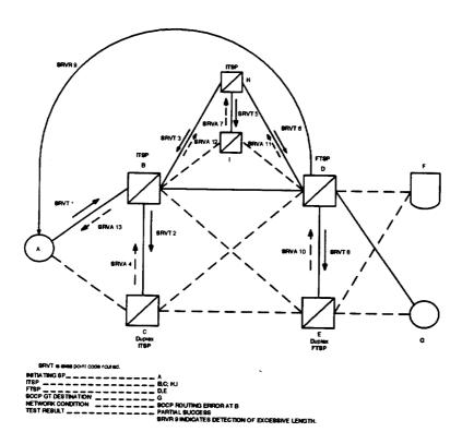
Figure 6-15. Detection of Excessive Length SCCP Route
