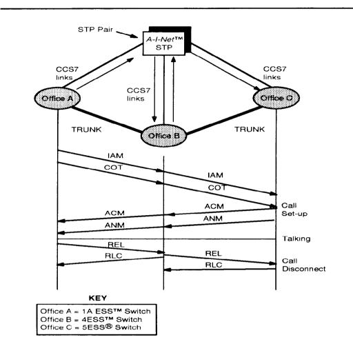
Figure 2-1. ISUP Call Processing in the SS7 Network
