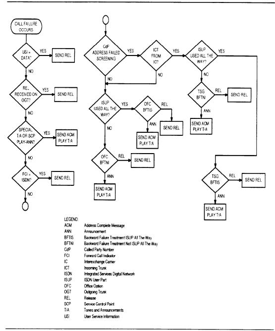
Figure 3-5. 4ESS Switch SS7 Call Failure Treatment at LEC Access Tandem (Incoming Trunk Is SS7)
