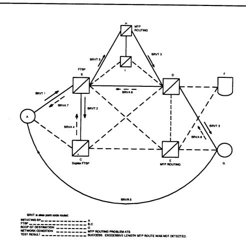
Figure 6-16. SRVT Does Not Detect Excessive Length, MTP Route
