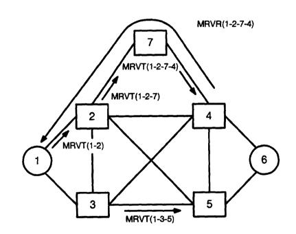
Figure 6-11. Example When Routing Loop Detected
