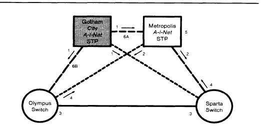
Figure 4-7. Example Network for A-1-Net Products STP Initialization
