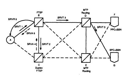
SRVT is alias point code routed. INITIATING SP\_\_\_\_\_\_ A FINAL TRANSLATION \_\_\_\_\_ B,C SCCP GT DESTINATION \_\_\_\_\_ F (PPC+SSN) NETWORK CONDITION \_\_\_\_\_ MTP ROUTING ERROR AT D SVRVT SENT TO G WHICH HAS PROCESSING DIFFICULTIES. TEST RESULT \_\_\_\_\_ PARTIAL SUCCESS. TIMER EXPIRED AT B WHILE WAITING FOR SRVA FROM F OR G.
