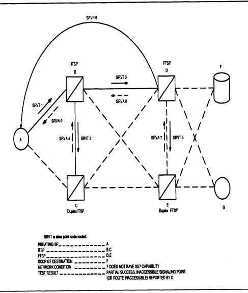
Figure 6-18. Inaccessible Signaling Point
