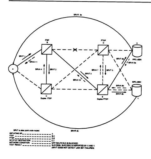
Figure 6-28. SRVT Bypasses Linkset Failure
