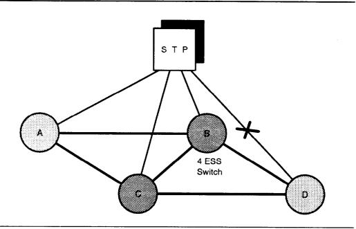
Figure 2-4. Direct Trunks to an End Office With Overflow to Another Local Tandem
