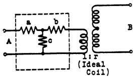
For Impedance at A: Divide the impedance connected at B by r (the impedance ratio of the coil involved, greater than 1)
