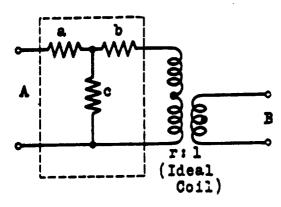
For Impedance at A: Multiply the impedance connected at B by r (the impedance ratio of the coil involved, greater than 1) and combine the resultant with the T-Network.
